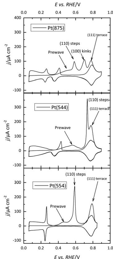
Fig. 8 CO stripping profiles for different stepped and kinked surfaces in 0.1 M NaOH. The arrows indicate the origin of the different peaks. Scan rate: 50 mV s<sup>-1</sup>.
