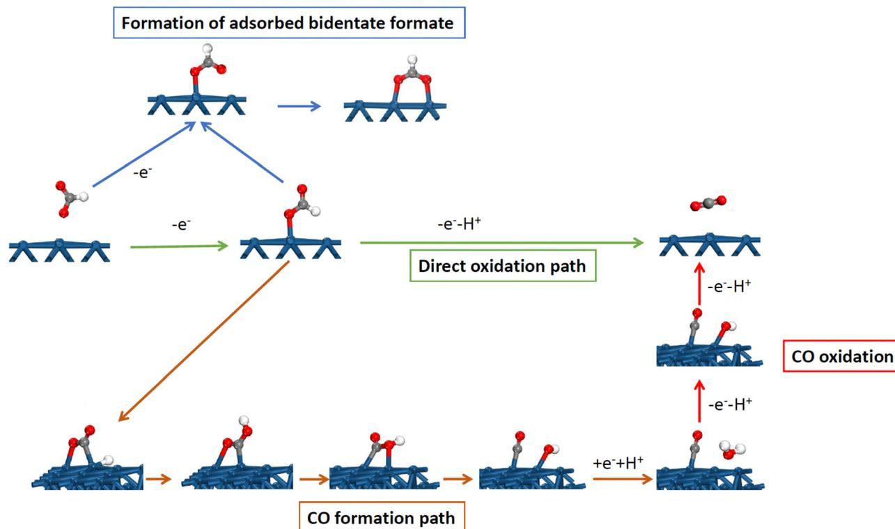
Fig. 6 Detailed mechanism for the formic acid oxidation reaction on platinum electrodes, showing the direct oxidation path, the path forming adsorbed CO and its oxidation, and the formation of bidentate adsorbed formate.
