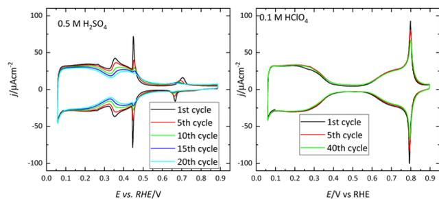
Fig. 2 Evolution upon cycling of the voltammetric profiles of a Pt(111) electrode in 0.5 M H<sub>2</sub>SO<sub>4</sub> and 0.1 M HClO<sub>4</sub> with different levels of impurities. Scan rate: 50 mV s<sup>-1</sup>.
