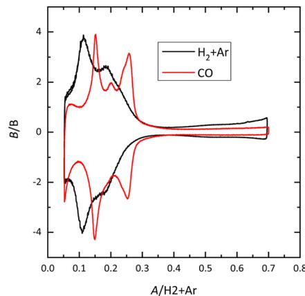
Fig. 4 Voltammetric profile for the Pt(110) electrode in 0.1 M HClO<sub>4</sub> cooled down in different atmospheres. Scan rate: 50 mV s<sup>-1</sup>.
