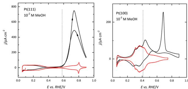
Fig. 7 Voltammetric profiles for the methanol oxidation reaction in 0.1 M HClO<sub>4</sub> (black curves) on Pt(111) and Pt(100) electrodes. The red curves show the profiles obtained in the absence of methanol and the vertical dashed lines represent the onset of OH adsorption on these surfaces. Scan rate: 50 mV s<sup>−1</sup>.
