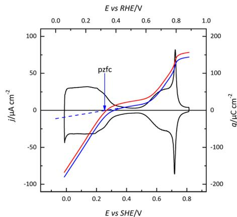
Fig. 5 Voltammetric profile (black line) of the Pt(111) electrode in 0.1 M HClO<sub>4</sub> and integration curves using the CO displaced charge displaced at 0.1 V before (red line) and after (blue line) correction for the residual charge of CO CO-covered electrode. The blue dashed line shows the extrapolation of the straight region to determine the pzfc.
