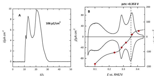
Fig. 3 (A) CO displaced charge at 0.24 V for the Pt(311) electrode in 0.1 M HClO<sub>4</sub>. (B) Voltammetric profile (left axis) and total charge curve (right axis) for the Pt(311) electrode in 0.1 M HClO<sub>4</sub>. The red points indicate the displaced charge used as integration constants for the charge curve. Scan rate: 50 mV s<sup>-2</sup>.
