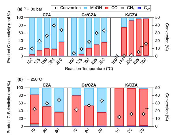
Fig. 4  $CO_2$  conversion (markers) and product selectivity (bars) of CZA, Ca/CZA, and K/CZA in the co-fed  $CO_2$  hydrogenation reaction at (a) T=150-250 °C at 30 bar and (b) P=10-30 bar at 250 °C. Reaction conditions: WHSV of 0.5  $g_{CO_2}$   $g_{cat}^{-1}$  h<sup>-1</sup> and  $H_2$ :  $CO_2$  molar ratio of 3:1. Materials were pre-reduced in 95%  $H_2$ /Ar for 16 h at 250 °C.
