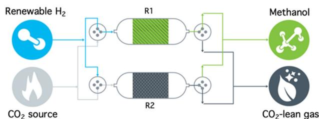
Fig. 1 Conceptualized process flow diagram of RCC-to-methanol.
