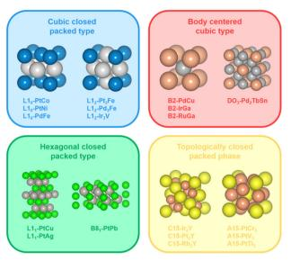
Fig. 1 Illustration of various crystal structures of intermetallic nanocatalysts
