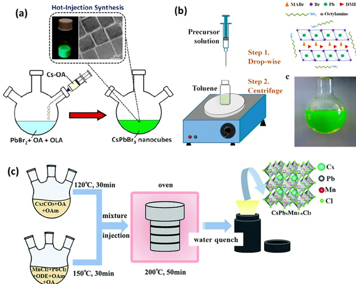
Fig. 2 Diagram depicting perovskite synthesis techniques: (a) hot injection,<sup>47</sup> (b) LARP,<sup>50</sup> and (c) solvothermal method.<sup>53</sup> Reproduced with permission from ref. 47 Copyright © 2022 American Chemistry Society. Reproduced with permission from ref. 50 Copyright © 2015 American Chemistry Society. Reproduced with permission from ref. 53 Copyright © 2018 Royal Society of Chemistry.
