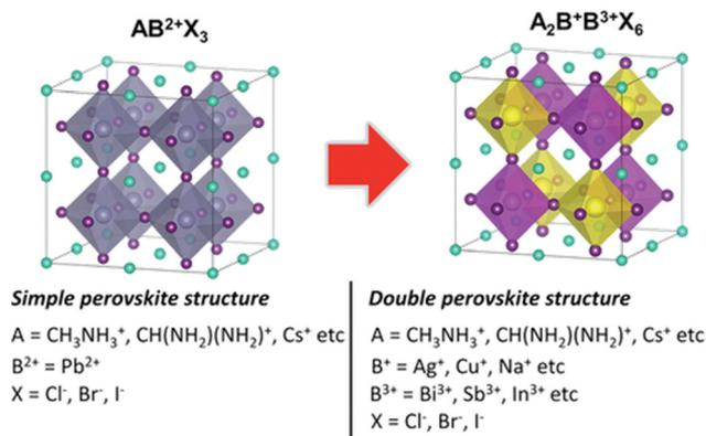
**Fig. 1** Illustration of structural contrasts between simple (AB<sup>2+</sup>X<sub>3</sub>) and double perovskites (A<sub>2</sub>B<sup>+</sup>B<sup>3+</sup>X<sub>6</sub>). Visualization of A<sup>+</sup>, B<sup>2+</sup>, B<sup>+</sup>, B<sup>3+</sup>, and X<sup>−</sup> ions depicted as cyan, gray, yellow, pink, and purple spheres, respectively.<sup>43</sup> Reproduced with permission from ref. 43 © 2019 Wiley-VCH Verlag GmbH & Co. KGaA, Weinheim.
