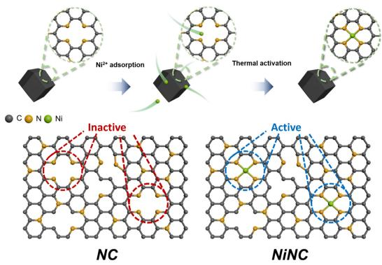
Fig. 1 Schematic illustration of the synthesis of the N-doped carbon (NIC) material and the single nickel atoms anchored on the N-doped carbon (NIC). The inert pyridinic nitrogen sites convert into electrochemically active sites through the introduction of single Ni atoms.
