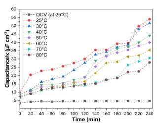
Fig. 7 Tracking the electrode flooding by DLC measurements as a function of the operating temperature at 200 mA cm<sup>-2</sup>. OCV was conducted at room temperature. Experimental conditions: Cu-GDE (Cathode), MPIP-AEM, IrO<sub>2</sub> (Anode), CO<sub>2</sub> flow rate: 20 sccm, 0.1 M KHCO<sub>3</sub> as anolyte.
