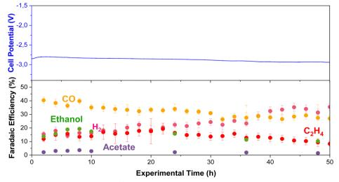
Fig. 9 Long-term stability test at 60  $^{\circ}$ C and 150 mA cm<sup>-2</sup> using Cu-electrocatalyst. Experimental conditions: Cu-GDE (Cathode), MPIP-AEM, IrO<sub>2</sub> (Anode), CO<sub>2</sub> feeding rate 20 sccm, 0.1 M KHCO<sub>3</sub> as anolyte. Error bars represent the standard error of different injections and measured samples.
