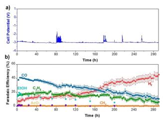
Fig. 10 290 hour  $CO_2$  electrolysis stability test at 60 °C and 200 mA cm<sup>-2</sup>. (a) Potential profile. (b) Faradaic efficiency. Operating parameters were sputtered Cu cathode with 10% be weight MPIP ionomer, MPIP membrane, IrO<sub>2</sub> on carbon anode and 0.1 M CsHCO<sub>3</sub> as an electrolyte. 100 mbar back pressure on the cathode was used as well. Error bars represent the standard error of different injections and measured samples.
