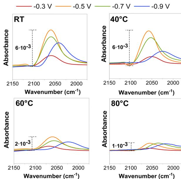
Fig. 2 ATR-SEIRAS  $\text{CO}$  adsorption peak for electrochemical  $\text{CO}$  reduction at different potentials (vs. RHE) and operating temperatures. The  $\text{CO}$  partial pressure for each operating temperature is detailed in Fig. S5 and S6 and estimated with eqn (S12) (ESI†).
