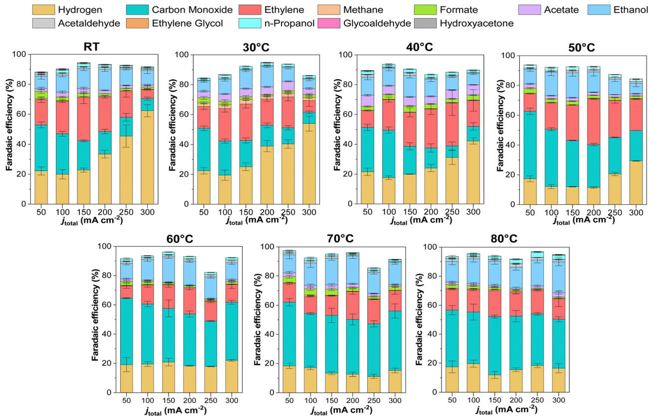
Fig. 5 Temperature effects on the product distribution for CO<sub>2</sub>R over Cu-based electrocatalysts using zero-gap configuration at different temperatures and current densities. Experimental conditions: Cu-GDE (Cathode), MPIP-AEM, IrO<sub>2</sub> (Anode), CO<sub>2</sub> feeding rate 20 sccm, 0.1 M KHCO<sub>3</sub> as anolyte. Error bars represent the standard error of the independent measurements at each different reaction condition.
