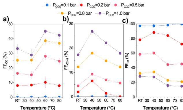
Fig. 6 Product distribution and faradaic efficiencies of gas products at different operating temperatures and partial pressures of CO<sub>2</sub> (diluted with Ar): (a) CO, (b) C<sub>2</sub>H<sub>4</sub>, and (c) H<sub>2</sub>. Experiments were conducted at 200 mA cm<sup>-2</sup>. Error bars represent the standard error of three independent measurements at each different condition.
