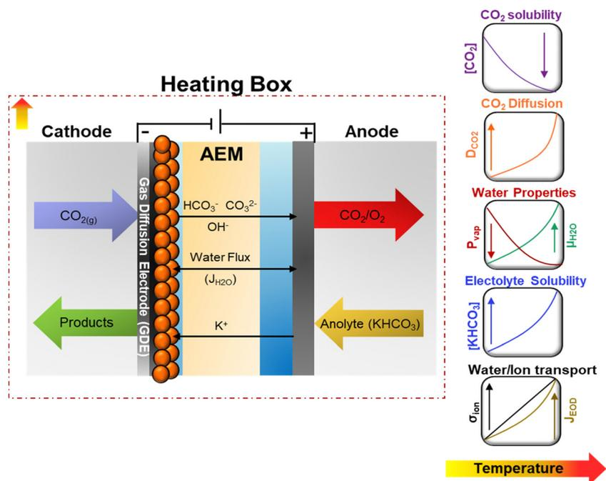
Fig. 1 Schematic representation of temperature dependency on transport and kinetics properties on  $CO_2E$  in zero-gap configuration. Equations for the presented trends for the different properties can be found in the ESI.†
