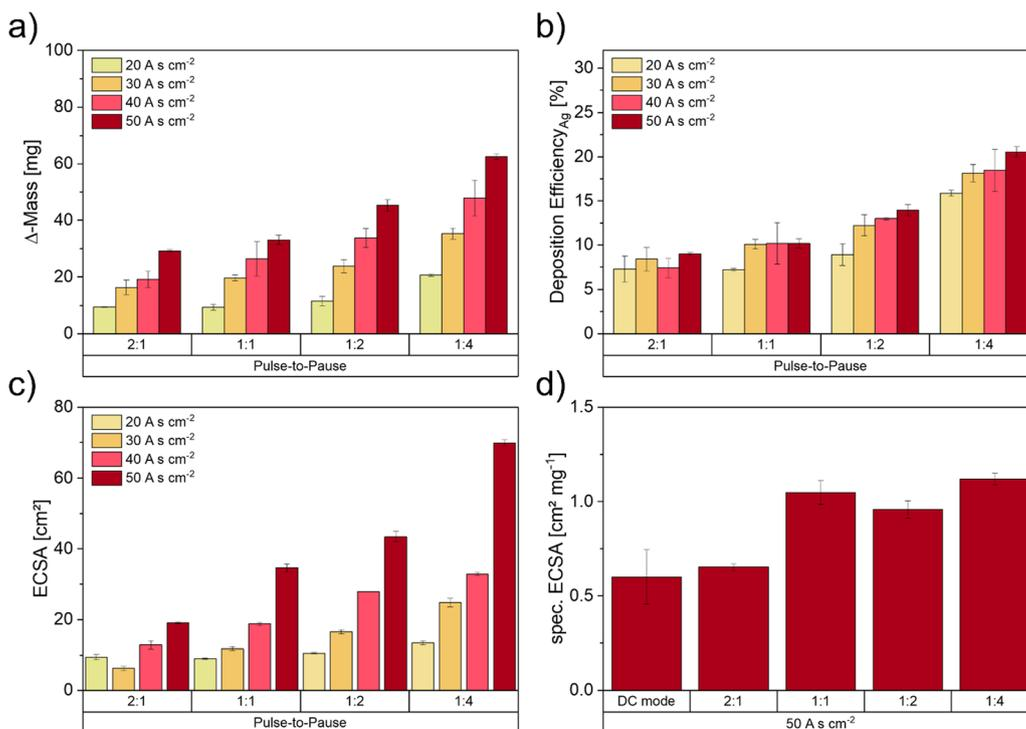
**Fig. 4** Electrochemically deposited masses (a) and the calculated FE of the DHBT in dependence of the varied pulse-to-pause ratios (b), calculated ECSA values by measurement of the double layer capacity and specific ECSA (d) of the deposited samples with 50  $\text{A s cm}^{-2}$  in dependence of the pulse-to-pause ratios.
