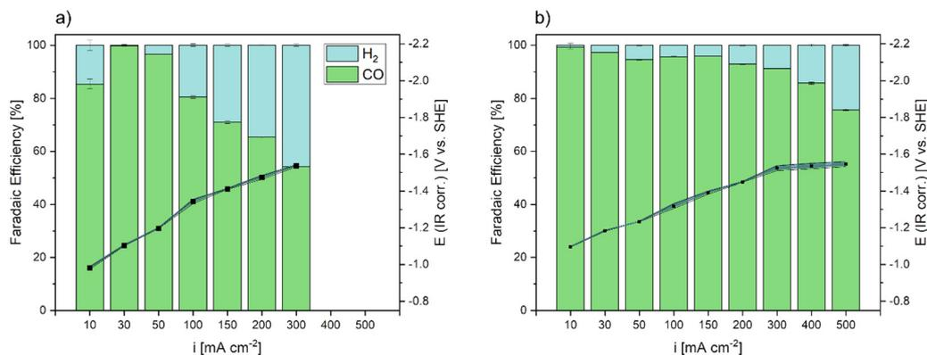
Fig. 8 Normalized faradaic efficiencies of CO and H<sub>2</sub> after galvanostatic operation at current densities up to 500 mA cm<sup>-2</sup> and the recorded WE potential after correction for the inner resistance. (a) CO<sub>2</sub>RR results of a commercial Covestro GDE and (b) CO<sub>2</sub>RR results of the Ag DHBT GDE. Each curve represents the mean of two replicate measurements with the respective standard deviations indicated by the shaded areas.
