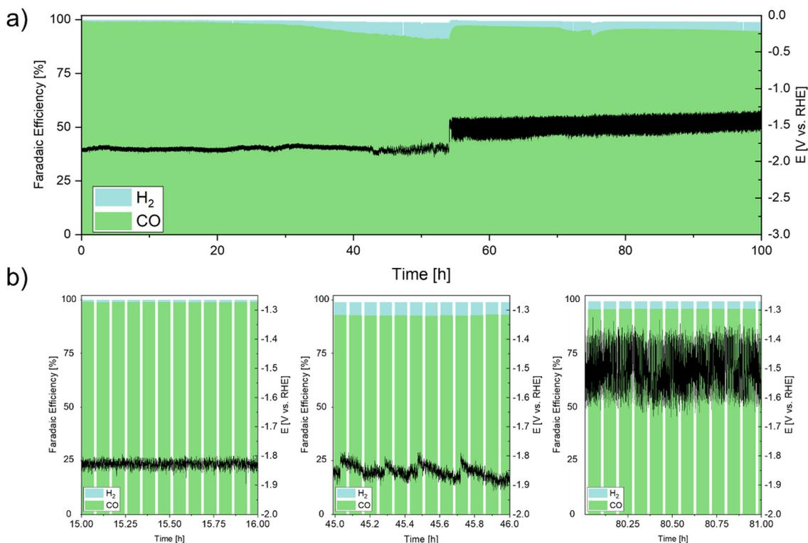
Fig. 9 Long-term stability tests of the DHBT-GDE in galvanostatic mode at 200 mA cm<sup>-2</sup> for 100 h. (a) WE potential without compensation and normalized FE of the only detected products over 100 h, (b) WE potential and FE of 1 h of operation each, during three different operating stages.
