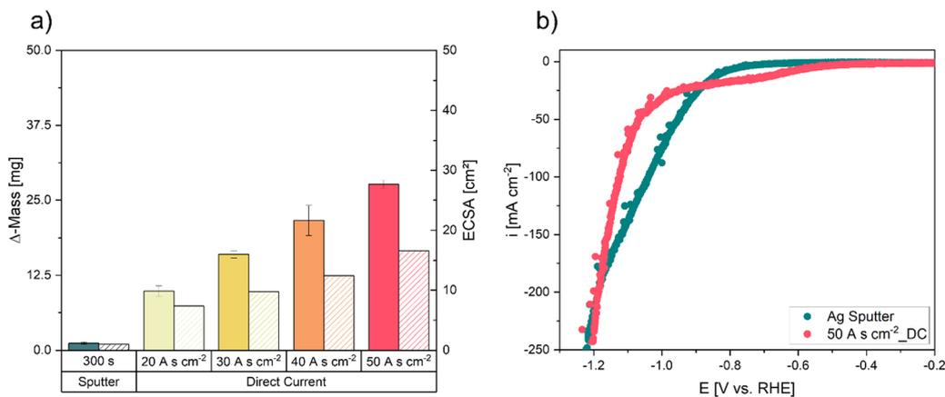
**Fig. 3** Characterization of the Ag-sputtered electrode compared to the DHBT electrodes manufactured in DC mode. (a) Deposited Ag mass and ECSA values of Ag-sputtered electrode and DHBT foam electrodes with increasing charge densities during DC mode, (b) linear sweep voltammetry curves for the Ag sputter electrode and the DC-50  $\text{A s cm}^{-2}$  electrode to test their electrochemical performance (IR corrected potentials by applied CI method).
