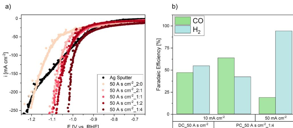
Fig. 5 Electrochemical performance of the electrodeposited electrodes compared to the sputtered electrode. (a) Linear sweep voltammetry measurements for GDEs deposited with a charge density of  $50\text{ A s cm}^{-2}$ , (b) faradaic efficiency of the detected  $CO_2RR$  products after 1 h of operation (b).
