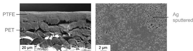
Fig. 1 Analysis of electrode microstructure by scanning electron microscopy. (a) Cross-section of a pristine polymer fibre fabric and (b) top-down view of the polymer substrate, which was sputtered with Ag for 360 s.
