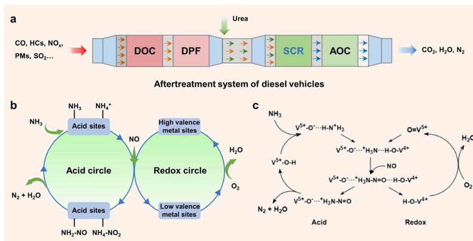
**Fig. 1** (a) The after-treatment system of diesel vehicles. (b) Efficient methods for enhancing the acid cycle and redox cycle over de-NO<sub>x</sub> catalysts. (c) The catalytic reaction diagram revealing the double cycles of the NH<sub>3</sub>-SCR process over vanadia/titania catalysts. Copied with permission from ref. 32. Copyright 1995, Elsevier.
