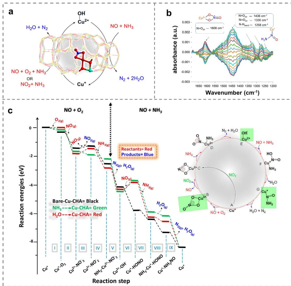
Fig. 3 (a) Schematic of the NH<sub>3</sub>-SCR reaction mechanism on Cu-SSZ-13 zeolites. (b) Concentration modulation ME DRIFTS experiment with the corresponding phase-resolved spectrum. (c) Reaction mechanisms on the bare active site (black), ammonia-physorbed active site (green) and water-physorbed active site (red). Copied with permission from ref. 76. Copyright 2022, American Chemical Society.
