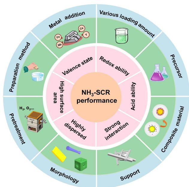
Fig. 2 Effect factors of  $\text{NH}_3$ -SCR activity.
