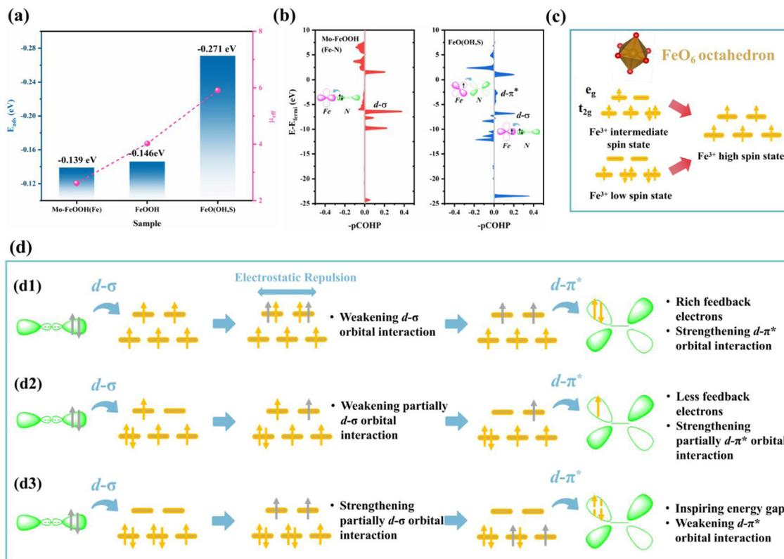
Fig. 6 (a) Spin states and  $N_2$  adsorption energies of Fe sites for different FeOOH-based catalysts; (b) the  $-pCOHP$  of Fe–N interactions and the electron donation-acceptance process between Fe sites and  $N_2$  for FeO(OH, S) and Mo–FeOOH; (c) spin states and corresponding d-orbital electronic structures of Fe sites; (d) the possible mechanisms of the spin state effect for the  $N_2$  activation process.
