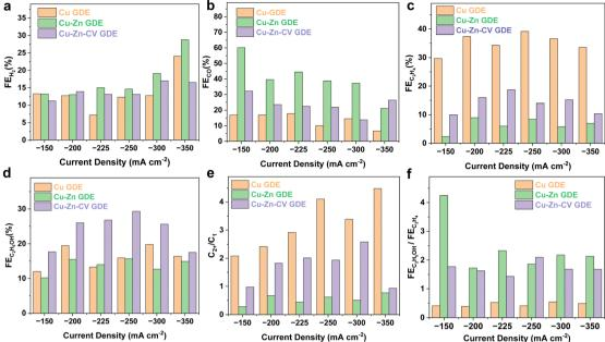
Fig. 5 Cu-GDE, Cu-Zn-GDE layered bimetallic catalyst, and Cu-Zn-CV-GDE catalysts in the current density range from -150 to -350 mA cm<sup>-2</sup>: (a) FE of  $H_2$ , (b) FE of CO, (c) FE of  $C_2H_4$ , and (d) FE of  $C_2H_5OH$ . (e) The ratio of FE towards  $C_2+$  to  $C_1$  products. (f) The ratio of FE towards  $C_2H_5OH$  to  $C_2H_4$ . products
