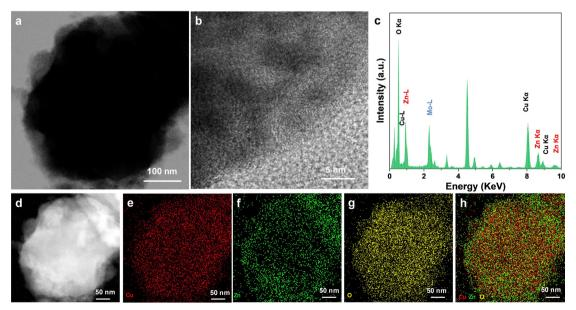
Fig. 4 (a) TEM image of the Cu-Zn-CV-GDE catalyst. (b) HRTEM image, (c) EDS image, (d) high-angle annular dark field scanning transmission electron microscopy (HADDF-STEM) image and (e)-(h) superposition image of Cu, Zn, O and three element mapping
