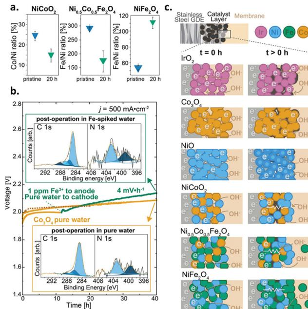
**Fig. 8** (a) Metal ratios before and after testing in pure water for bimetallic oxide catalysts measured with XPS. (b) The role of solvated iron species in single-cell degradation, where Fe-spiked water showed increased oxidation of the ionomer *vs.* pure water evidenced with XPS (inserts). (c) Proposed mechanism of single-cell degradation for six oxide catalysts. Reprinted with permission from Krivina *et al.*, *Advanced Materials*, Copyright (2022) John Wiley and Sons.<sup>54</sup>
