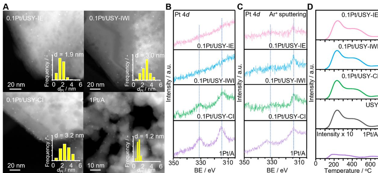
Fig. 1 (A) HADDF-STEM images and corresponding Pt size distribution of 0.1Pt/USY prepared with different methods and 1Pt/A; Pt 4d XPS spectra (B) before and (C) after Ar ion sputtering of 0.1Pt/USY prepared with different methods and 1Pt/A; (D) NH<sub>3</sub>-TPD profile of 0.1Pt/USY prepared with different methods, pristine USY and 1Pt/A.
