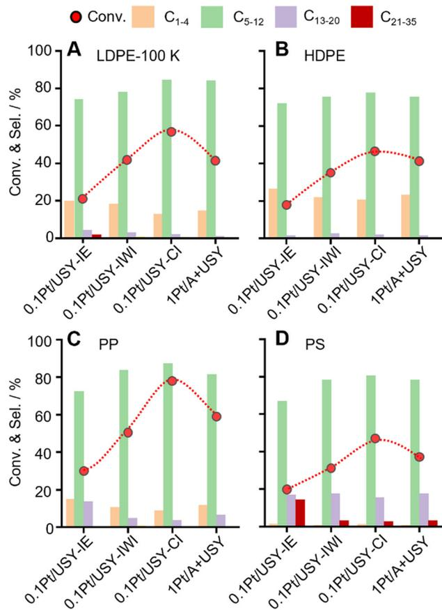
Fig. 6 Hydrocracking of various polyolefins over Pt-USY catalysts with different metal-acid proximity. (A) LDPE-100K ( $M_w = 100$  kDa); (B) HDPE ( $M_w = 142$  kDa); (C) PP ( $M_w = 27$  kDa); (D) PS ( $M_w = 4.6$  kDa). Reaction conditions: polyolefins, 4.0 g, catalyst, 0.2 g (for 0.1Pt/USY) or 1Pt/A + USY, 0.02 + 0.2 g, 280 °C, 3 MPa  $\text{H}_2$ , 3 h.
