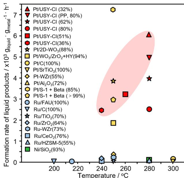
Fig. 8 Comparison of the formation rate of liquid products of various catalysts for the hydrocracking and hydrogenolysis of polyolefins. The data in brackets indicate the conversion of substrate PE or PP.
