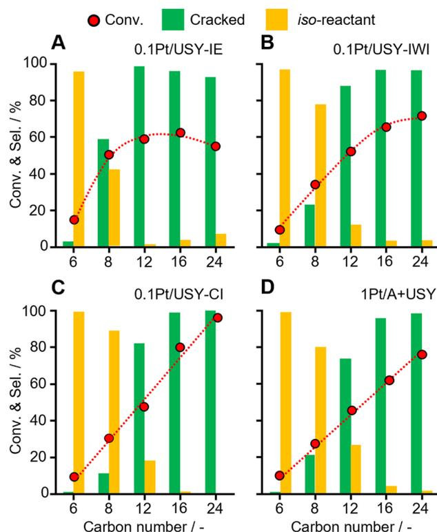
Fig. 4 Hydrocracking different *n*-alkanes over Pt-USY catalysts with various metal-acid proximity. (A) 0.1Pt/USY-IE; (B) 0.1Pt/USY-IWI; (C) 0.1Pt/USY-CI and (D) 1Pt/A + USY. Reaction conditions: *n*-alkanes, 4.0 g, catalyst, 0.2 g (for A–C) or 1Pt/A + USY, 0.02 + 0.2 g (for D), 240 °C, 3 MPa  $\text{H}_2$ , 3 h.
