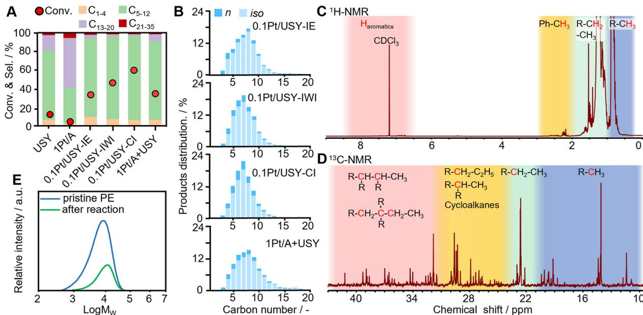
Fig. 3 (A) Catalytic performance of Pt-USY with different metal-acid proximity and referential catalysts in hydrocracking PE; (B) product distribution of the corresponding Pt-USY catalysts; (C)  $^1\text{H-NMR}$  and (D)  $^{13}\text{C-NMR}$  spectra profile of typical liquid products; (E) molecular weight distributions of pristine PE and solid product by HT-GPC. Reaction conditions: PE, 4.0 g, catalyst, 0.2 g (for 0.1Pt/USY) or 1Pt/A + USY, 0.02 + 0.2 g, 280 °C, 3 MPa  $\text{H}_2$ , 3 h.
