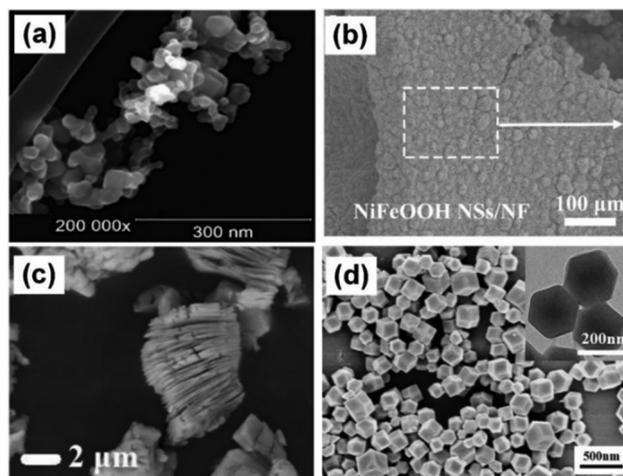
Fig. 3 Morphology of photocatalysts for bioaerosol inactivation. (a) TiO<sub>2</sub> nanoparticles,<sup>56</sup> Reproduced with permission. Copyright 2019, Elsevier. (b) NiFeOOH nanosheets,<sup>75</sup> Reproduced with permission. Copyright 2023, Elsevier. (c) MXene,<sup>63</sup> Reproduced with permission. Copyright 2021, Elsevier. (d) MOF (ZIF-8),<sup>85</sup> Reproduced with permission. Copyright 2022, Elsevier.
