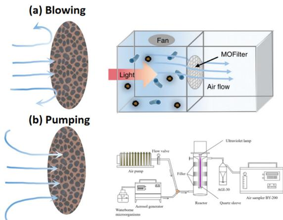
Fig. 13 Performance evaluations of bioaerosol capture. (a) Bioaerosol blowing,<sup>64</sup> reproduced with permission. Copyright 2019, Nature Publishing Group. (b) Bioaerosol pumping,<sup>38</sup> reproduced with permission. Copyright 2022, Elsevier.
