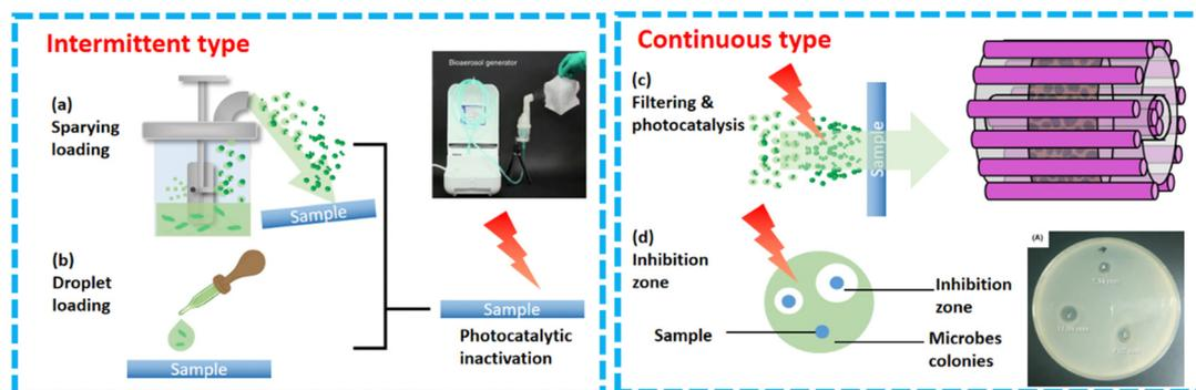
Fig. 14 Performance evaluations of bioaerosol inactivation. (a) Spraying loading with following irradiation.<sup>64</sup> Reproduced with permission. Copyright 2019, Nature Publishing Group. (b) Droplet loading with the following irradiation. (c) Filtering and photocatalysis. (d) Inhibition zone.<sup>127</sup> Reproduced with permission. Copyright 2019, Wiley-VCH GmbH.
