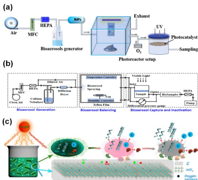
Fig. 11 The wavelength utilized by photocatalysts. (a) UV,<sup>75</sup> reproduced with permission. Copyright 2023, Elsevier. (b) Visible light,<sup>105</sup> reproduced with permission. Copyright 2023, Elsevier. (c) Infrared,<sup>171</sup> reproduced with permission. Copyright 2020, American Chemical Society.
