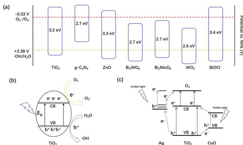
Fig. 5 The mechanism of light-induced reactive oxygen species by semiconductor photocatalysts. (a) Bandgaps of some typical semiconductors. Charge separation of (b) TiO<sub>2</sub> and (c) Cu and Ag doped TiO<sub>2</sub>.
