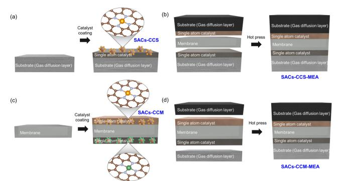
Schematic of (a) SAC-CCS-MEA and (b) MEA fabrication by hot pressing. (c) Schematic of the SAC-CCM-MEA and (d) MEA fabrication.
