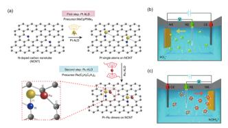
(a) Schematic of synthesis process of the Pt-Ru dimer SACs using ALD process. Reproduced with permission from ref. 179. Copyright 2019, Springer Nature. Schematics of (b) cathodic and (c) anodic deposition of Ir species using three-electrode system. Reproduced with permission from ref. 187. Copyright 2020. Springer Nature.
