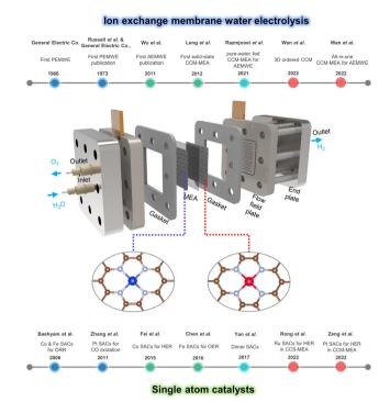
Fig. 1 Schematic illustration of SACs-incorporated MEA water electrolyzer and timelines of developments in ion exchange membrane water electrolyzer and single atom catalysts.
