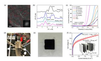
Fig. 13 (a) HAADF-STEM image of Pt<sub>1</sub>/CoHPO showing the isolated Pt single atoms. The normalized EXAFS spectra of Pt foil, PtO2, Pt(OH4)-2H2O and Pt<sub>1</sub>/CoHPO. (c) Polarization curves of the OER catalysts. Digital photograph of (d) AEMWE device and (e) CCM-type MEA. (f) I-V curves of AEMWE device using benchmark Pt/C||Ir/C and Pt<sub>1</sub>/CoHPO. Reproduced with permission from ref. 104. Copyright 2022. Springer Nature.
