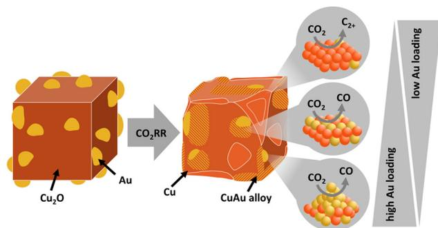
Fig. 7 Schematic illustration of the catalyst structure in the as-prepared state and during/after the  $\text{CO}_2\text{RR}$ , with their corresponding main products. The triangles indicate the amount of Au loading favoring the different Au–Cu atomic structures/redistributions.
