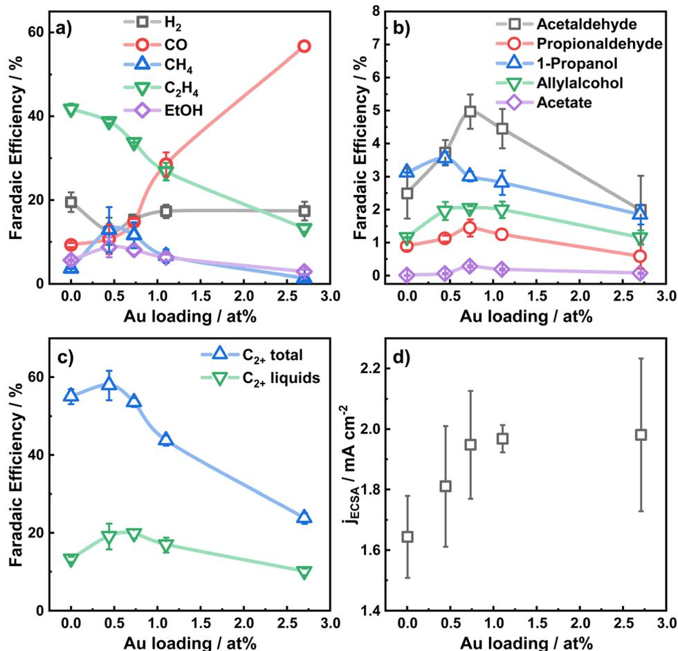
Fig. 2 Faradaic efficiencies at  $-1.07$  V in 0.1 M KHCO<sub>3</sub> as a function of the Au NP loading for (a) H<sub>2</sub>, CO, CH<sub>4</sub>, C<sub>2</sub>H<sub>4</sub>, (b) minor liquid products, (c) C<sub>2+</sub> total products, C<sub>2+</sub> liquid products; (d) Au-loading dependency of the current density normalized by the electrochemical surface area.
