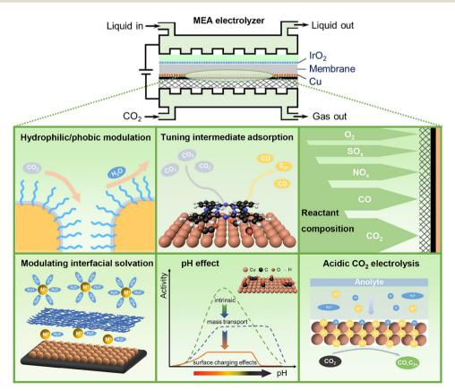
Fig. 1 Reaction microenvironment control in MEA electrolyzers for CO<sub>2</sub> electrolysis
