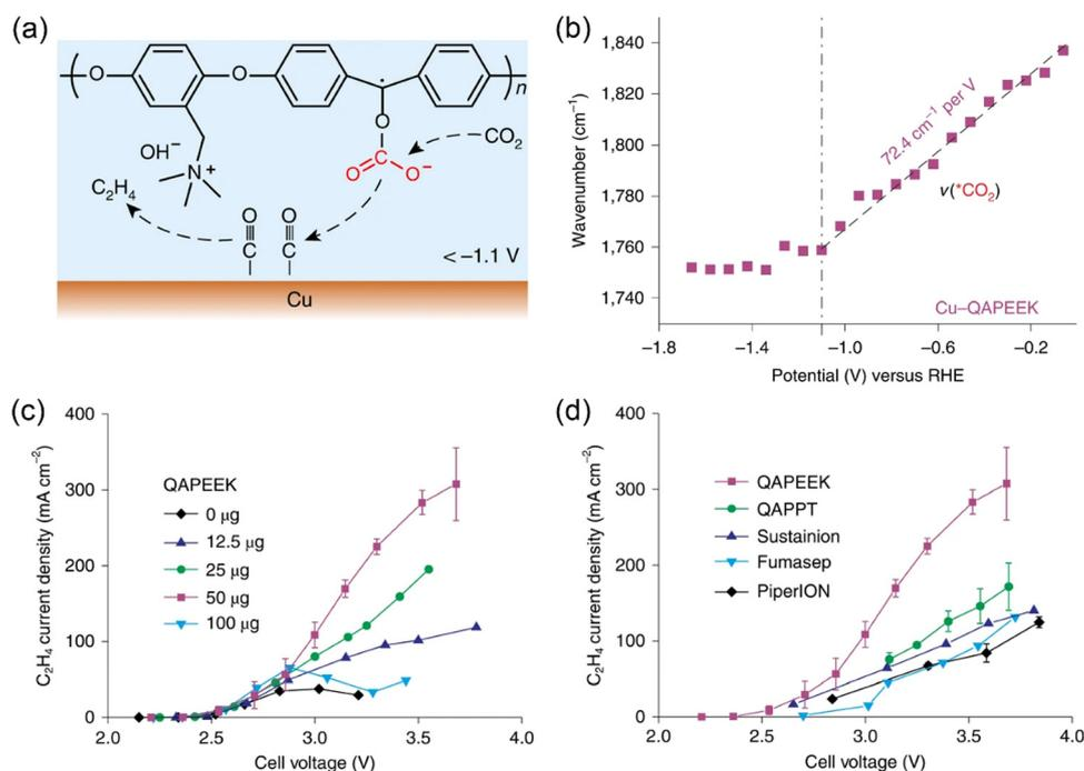
Fig. 3 (a) Schematic illustration of QAPEEK-promoted CO<sub>2</sub> electroreduction on Cu. (b) Potential-dependent shift of ATR-SEIRAS band of activated CO<sub>2</sub> (\*CO<sub>2</sub>) on Cu-QAPEEK. (c, d) Ethylene partial current densities of (c) Cu-QAPEEK electrodes with different amounts of QAPEEK and (d) Cu electrodes with different ionomers. Reproduced with the permission.<sup>61</sup> Copyright 2022, Springer Nature.
