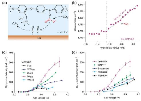
Fig. 3 (a) Schematic illustration of QAPEEK-promoted  $CO_2$  electroreduction on Cu. (b) Potential-dependent shift of ATR-SEIRAS band of activated  $CO_2$  (\*CO<sub>2</sub>) on Cu-QAPEEK. (c, d) Ethylene partial current densities of (c) Cu-QAPEEK electrodes with different amounts of QAPEEK and (d) Cu electrodes with different ionomers. Reproduced with the permission.<sup>61</sup> Copyright 2022, Springer Nature.
