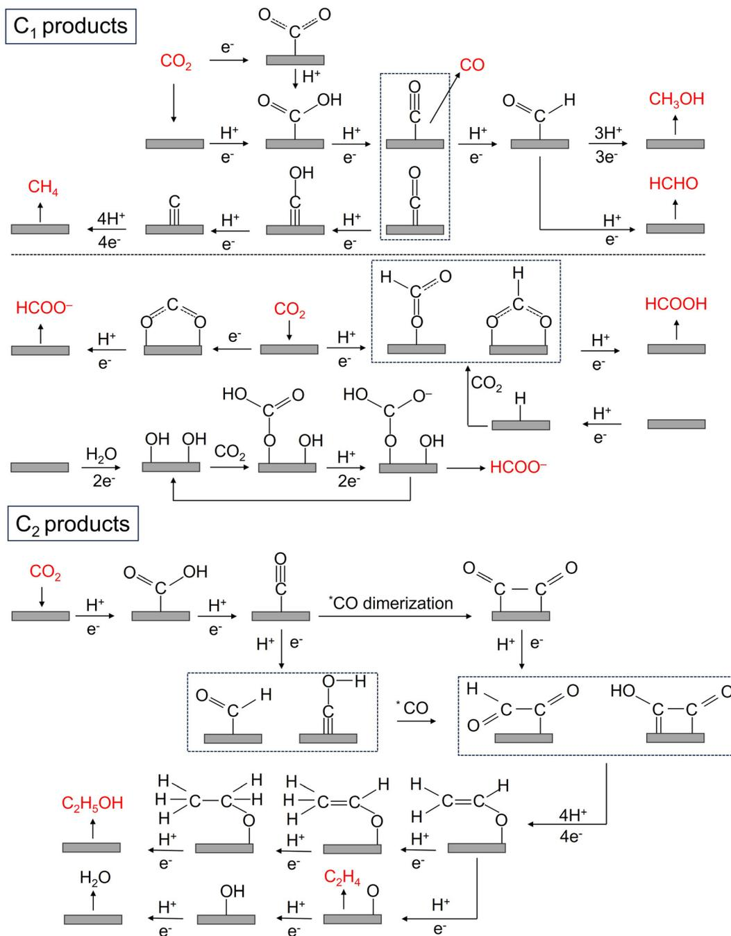
Fig. 3 The possible reaction pathways of C<sub>1</sub> and C<sub>2</sub> products in the CO<sub>2</sub>RR.
