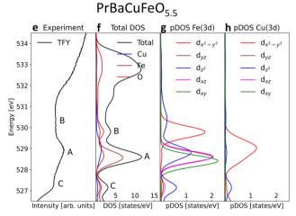
Fig. 7 Comparison between the O K-edges measured in TFY mode and the DOS from DFT calculations together with the Fe, Cu and O partial-DOS and the contributions of the different empty Fe and Cu 3d orbitals. (a)-(d) LuBaCuFeO<sub>5</sub>. (e)-(h) PrBaCuFeO<sub>5.5</sub>.
