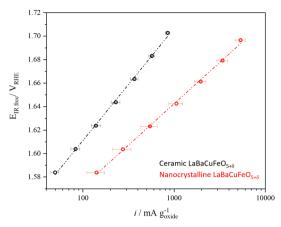
Fig. 9 Comparison between the gravimetric activity of the ceramic and nanocrystalline LaBaCuFeO<sub>5+δ</sub> samples.
