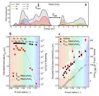
Fig. 8 (a) Calculated DOS for PrBaCuFeO<sub>5</sub> showing the location of the valence band O 2p centroid  $E_{cent}$  and the band gap  $E_{gap}$ . (b) Left axis: calculated Eqap for the RBaCuFeO<sub>5</sub> and RBaCuFeO<sub>6</sub> bulk materials. Right axis: experimental resistivity. (c) Comparison between the changes in the experimental OER activity upon R-cation replacement with those in the calculated valence band O 2p E<sub>cent</sub> for RBaCuFeO<sub>5</sub> and RBaCuFeO<sub>6</sub>.
