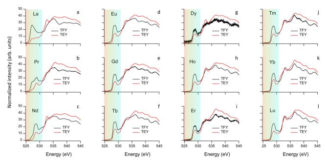
Fig. 6 O K-edges of RBaCuFeO<sub>5+ $\delta$ </sub> layered perovskites measured using the TFY and TEY modes. The color-shaded areas indicate the energy range associated to empty 3d TM states hybridized with the O 2p states.
