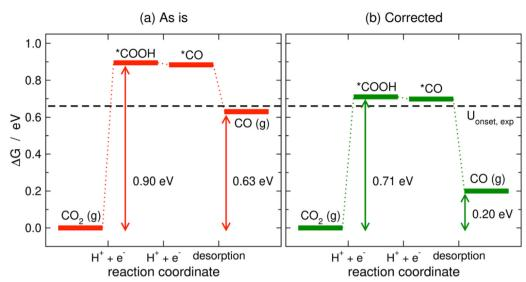
Fig. 11 PBE-calculated free-energy diagrams of the CO<sub>2</sub>RR to CO on Au(111) without (a) and with (b) gas-phase corrections. The Gibbs energies corresponding to the onset and equilibrium potentials are shown in each case along with the experimental onset potential (dashed line). Reproduced from ref. 34, licensed under CC-BY-NC-ND (https://creativecommons.org/licenses/by-nc-nd/4.0/).
