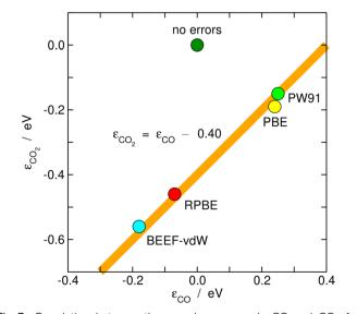
Fig. 7 Correlation between the gas-phase errors in CO and CO2 for various xc-correlation functionals. The hypothetical perfect agreement between DFT and experimental values is marked in dark green.
