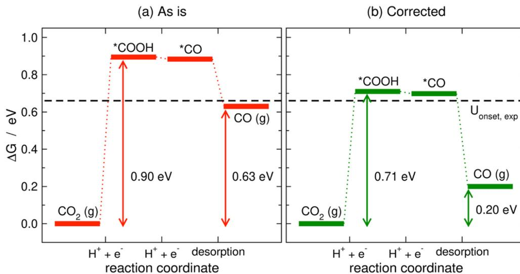
Fig. 11 PBE-calculated free-energy diagrams of the CO<sub>2</sub>RR to CO on Au(111) without (a) and with (b) gas-phase corrections. The Gibbs energies corresponding to the onset and equilibrium potentials are shown in each case along with the experimental onset potential (dashed line). Reproduced from ref. 34, licensed under CC-BY-NC-ND (<https://creativecommons.org/licenses/by-nc-nd/4.0/>).
