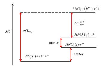
Fig. 8 Gibbs energy scale for HNO<sub>3</sub> relating the free energies of different states. Reproduced from ref. 51 Copyright 2013, Royal Society of Chemistry.
