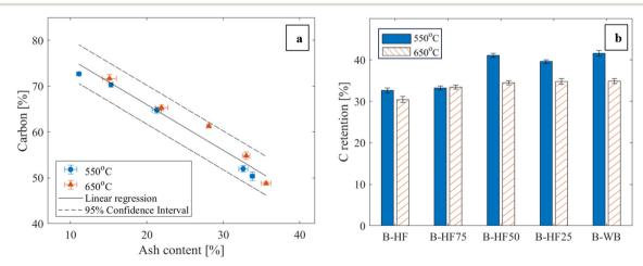
Fig. 7 Correlation between carbon and ash content (%) (a); and carbon retention (%) results (b) for biochars B-HF, B-HF50 and B-HF25. Carbon retention results calculated based on eqn (1). Error bars note the standard deviation of measured values (n = 3).
