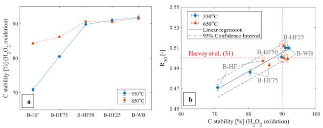
Fig. 6 Carbon stability (%) ( $H_2O_2$  oxidation method) for biochars B-HF, B-HF75, B-HF50, B-HF25 and B-WB produced at 550 °C, 650 °C (a); and correlation with the results of the  $R_{50}$  recalcitrance index method (b). Error bars note the standard deviation of measured values (n = 3).
