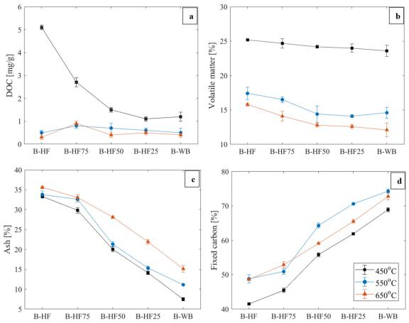
Fig. 3 Dissolved organic carbon (DOC) (a) and proximate analysis results (volatile matter (b), ash (c) and fixed carbon (dl)) for biochars B-HF, B-HF75, B-HF50, B-HF25 and B-WB produced at 450 °C, 550 °C, 650 °C (on a dry basis). Error bars note the standard deviation of measured values
