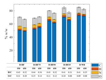
Fig. 4 CHN(S)O results, and calculated H/C and O/C molar ratios for biochars B-HF, B-HF75, B-HF50, B-HF25 and B-WB produced at 550, 650 °C (on a dry basis). The measured S values were  $\leq$  0.2% for all the samples and are not shown at this scale. Error bars note the standard deviation of measured values (n = 3)
