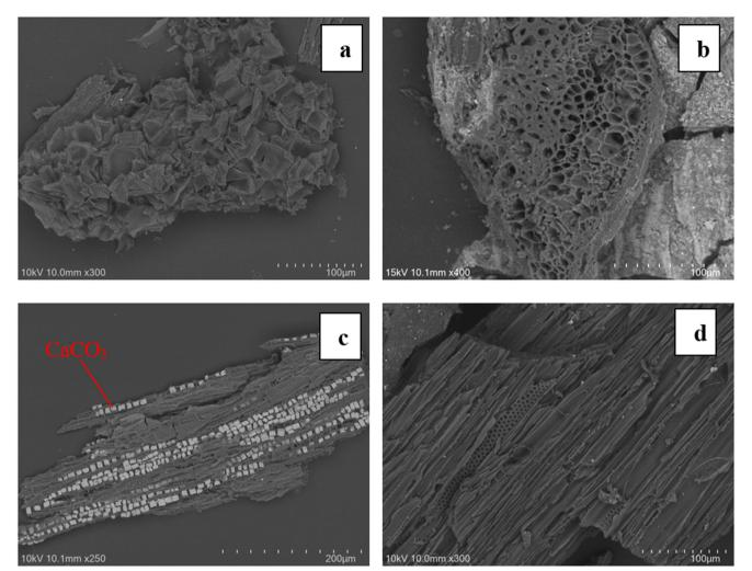
Fig. 5 Characteristic scanning electron microscopy (SEM) images for biochars B-HF (a), B-HF50 (b), B-HF50 (c) and B-HF25 (d) produced at 550 CaCO<sub>3</sub> precipitates identified via energy dispersive X-ray spectroscopy (EDX).
