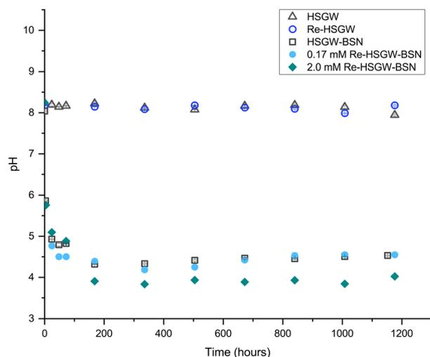
Fig. 1 Change of pH with time in the 0.17 mM and 2.0 mM  $\text{ReO}_4^-$  series with 0.1 g BSN starting material in 100 mL HSGW simulant. Control series: HSGW – groundwater simulant only; Re-HSGW – 0.17 mM Re in the simulant; HSGW-BSN – 100 mL groundwater simulant only; Re-HSGW – 0.17 mM Re in the simulant; HSGW-BSN – 100 mL groundwater simulant and 0.1 g BSN starting material. Error bars within the symbols are  $\pm 1$  st. dev. of triplicate measurements.
