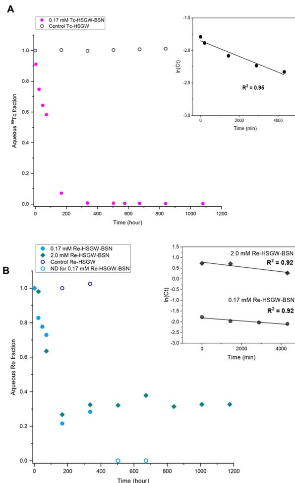
Fig. 2 Kinetics of  $\text{TcO}_4^-$  and  $\text{ReO}_4^-$  removal with BSN starting material (0.1 g) in HSGW simulant (100 mL). A. Removal of 0.17 mM  $\text{TcO}_4^-$ . Control series: 0.17 mM  $\text{TcO}_4^-$  in HSGW simulant. B. Removal of 0.17 and 2.0 mM  $\text{ReO}_4^-$ . Control series: 0.17 mM  $\text{ReO}_4^-$  in HSGW simulant (only select time points were analyzed). Insets: First order linear models for 72 hours (4320 min). ND – not detected (ICP-MS EQL for Re was 0.027 mM).
