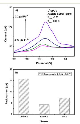
Fig. 8 (a) SWASV voltammograms of L<sup>1</sup>/SPCE registered in an acetate buffer solution containing a low concentration of Pb(II) ions; conditions: pH = 9.0,  $E_{\rm dep}$  = -1.0 V, and  $t_{\rm dep}$  = 600 s. (b) Response of the bare and modified-SPCE sensor to Cd ions.
