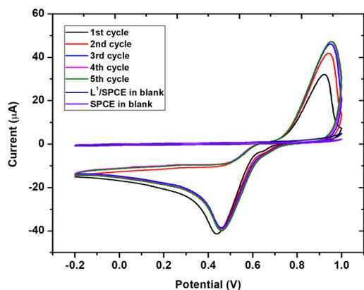
Fig. 9 Electrodeposition of AuNPs on  $L^1$ /SPCE using the cyclic voltammetry (CV) technique.
