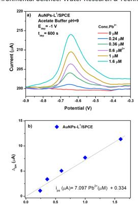
Fig. 10 SWASV voltammograms on (a) AuNPs-L<sup>1</sup>/SPCE in an acetate buffer solution containing a low concentration of Pb( $_{\rm II}$ ) ions; conditions: pH = 9.0,  $E_{\rm dep}$  = -1.0 V, and  $t_{\rm dep}$  = 600 s. (b) Calibration curve.
