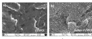
Fig. 5 High-resolution SEM images of the  $L^1$  sample without (a) and with AuNPs (b).
