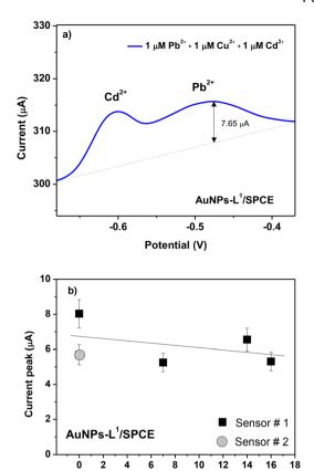
Fig. 12 (a) Selectivity test of the various HMI ions (Pb2+, Cu2+, and Cd<sup>2+</sup>) at 1 µM in seawater and (b) reproducibility test of two AuNPs-L<sup>1</sup>/ SPCE sensors and signal stability test up to 16 days.
