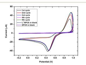
Fig. 9 Electrodeposition of AuNPs on L<sup>1</sup>/SPCE using the cyclic voltammetry (CV) technique.
