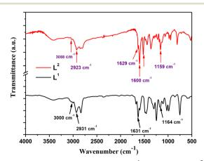
Fig. 1 FT-IR spectra of Schiff base ligands  $L^1$  (black line) and  $L^2$  (red line).
