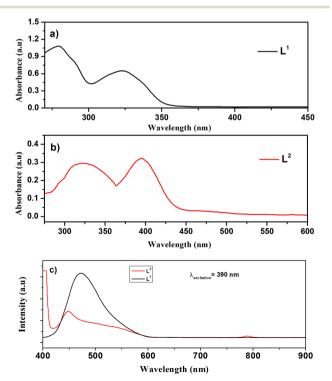
Fig. 3 UV-visible spectra of (a) L<sup>1</sup> and (b) L<sup>2</sup> ligands. (c) PL spectra of the Schiff base ligands; L1 (black line) and L2 (red line).
