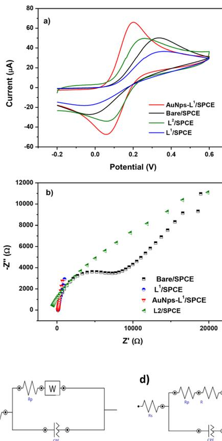
Fig. 6 (a) CV test, (b) Nyquist plots in  $[Fe(CN)_6]^{3-/4-}$  solution for bare/SPCE (black line),  $L^1$ /SPCE (blue line),  $L^2$ /SPCE (green line), and AuNPs- $L^1$ /SPCE (red line) electrodes. (c) The equivalent circuits of bare/SPCE,  $L^1$ /SPCE, and  $L^2$ /SPCE electrodes and (d) AuNPs- $L^1$ /SPCE.
