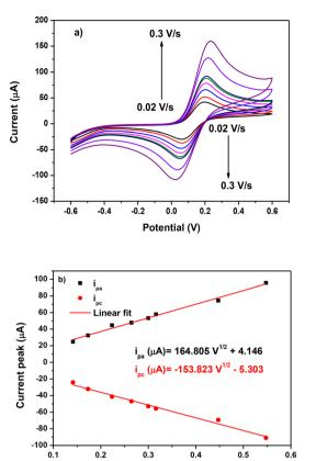
Fig. 11 (a) Scan rate variation study on AuNPs-L<sup>1</sup>/SPCE and (b) linearity of the  $i_p$  current peak vs. scan rate square root.
