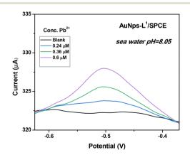
Fig. 13 Square-wave anodic stripping voltammograms (SWASVs) in seawater. Conditions:  $t_{\rm dep}$  = 600 s and  $V_{\rm dep}$  = -1 V.
