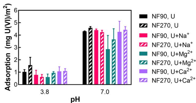
Fig. 4 Comparison of uranium(vi) adsorption by NF90 and NF270 at membrane iso-electric point (~3.8) versus neutral pH (~7.0). All solutions in these tests contained 150 μg L<sup>-1</sup> of uranium (added as UO<sub>2</sub>(NO<sub>3</sub>)<sub>2</sub>·6H<sub>2</sub>O) and were conducted at 22 °C. pH adjustments were made using 2% HNO<sub>3</sub> and 1 mM NaOH. Error bars are included to describe the standard error of the mean.
