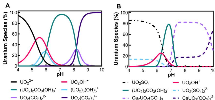
**Fig. 2** Uranium speciation modeling using Visual Minteq 3.1 2019 (Stockholm, Sweden). Both computations simulated an open system with carbonate at atmospheric concentrations ( $0.38 \times 10^{-3}$  atm  $\text{CO}_2$ ). A) Open system uranyl speciation with uranium concentration of 150  $\mu\text{g L}^{-1}$ , B) open system uranyl speciation with uranium concentration of 150  $\mu\text{g L}^{-1}$  and  $\text{CaSO}_4$  1  $\text{g L}^{-1}$ .
