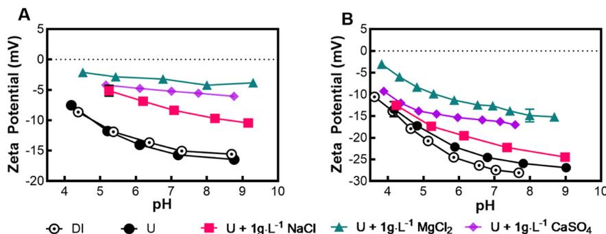
Fig. 1 Streaming zeta potential (mV) scans over pH ranges for A) NF90 and B) NF270 membranes. Additional tests included the addition of ions:  $\text{UO}_2(\text{NO}_3)_2 \cdot 6\text{H}_2\text{O}$ , NaCl,  $\text{MgCl}_2$ , and  $\text{CaSO}_4$ .
