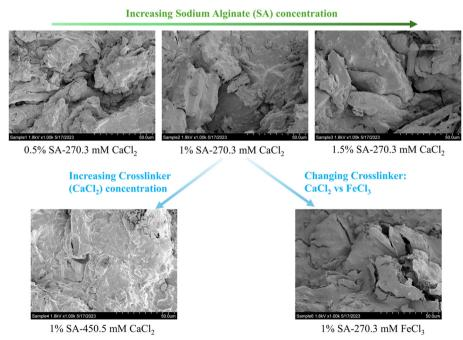
Fig. 3 Effects of varying bead compositions on the bead surface (SEM image scale bar =  $50 \mu m$ ). Increasing sodium alginate concentration smoothed the bead surface (crosslinker concentration was constant). Increasing the crosslinker concentration (3% to 5% CaCl<sub>2</sub>) or changing the crosslinker to FeCl<sub>3</sub> from CaCl<sub>2</sub> also smoothed the bead surface (sodium alginate concentration was constant). Large cracks and pores were evident in beads crosslinked with FeCl3.
