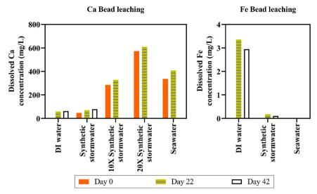
Fig. 5 Dissolved calcium concentration [leaching from Ca beads] and dissolved iron concentration [leaching from Fe beads] in solutions with different ionic strength (n = 1).  $10 \times$  synthetic stormwater,  $20 \times$  synthetic stormwater, and synthetic seawater data could not be collected on day 42.
