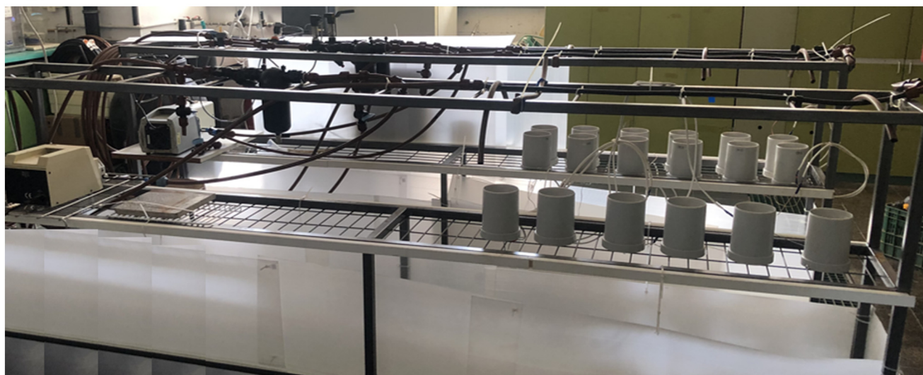
Fig. 2 a. Schematic of the laboratory pilot-scale drip irrigation rig; b. the laboratory pilot-scale drip irrigation rig.
