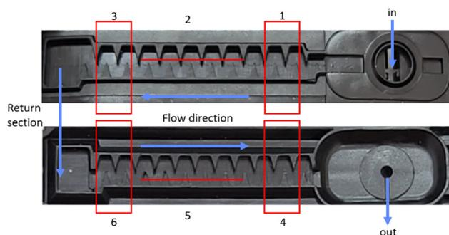
**Fig. 3** Internal image of the geometric channel of the drippers and the six sections scanned by OCT. Blue arrows indicate the flow direction. Areas 1,3,4 and 6 were 3D scanned and areas 2 and 5 were 2D scanned.
