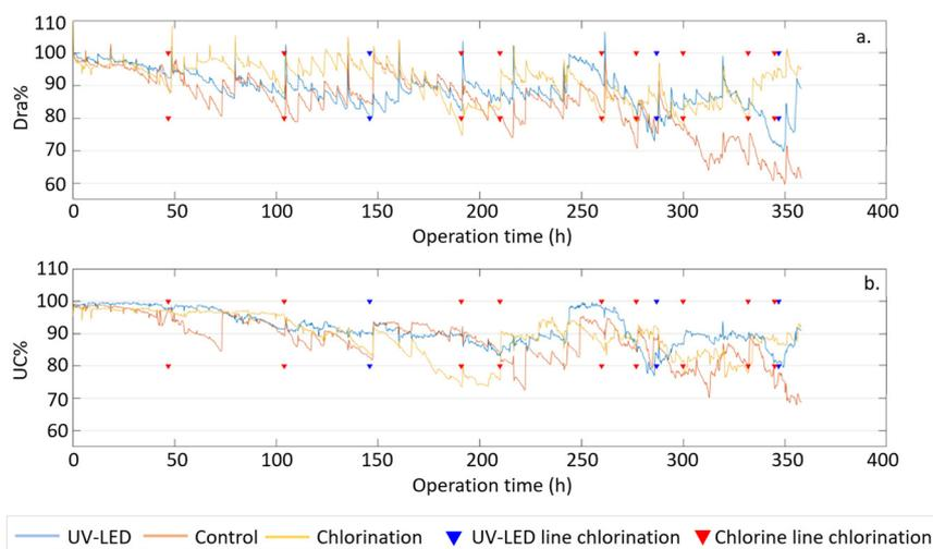
**Fig. 6** Analysis of flow through the dripper lines: a) relative overall drip emitter discharge along the line (Dra) vs. operation time. b) Uniformity coefficient (UC) vs. operation time. Triangles – maintenance of the pipelines by proactive chlorination.
