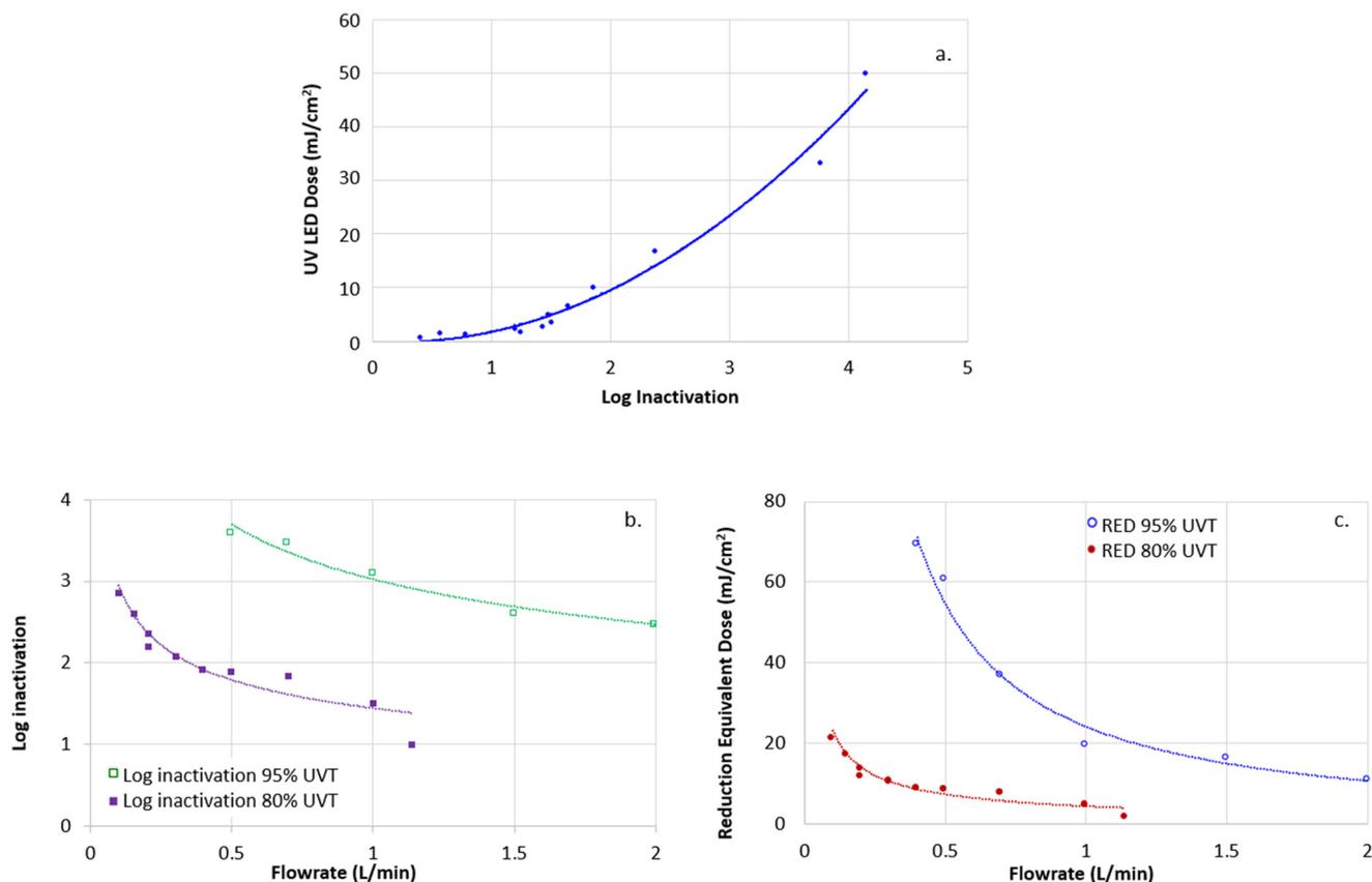
**Fig. 5** RED calculated by biosimetry. a. UV-LED dose response curve for the STWW solution (UVT 80%): log inactivation vs. UV-LED dose at the collimated beam apparatus; b. log inactivation of the UV-LED flow-through reactor in two different solutions (UV transmittance); c. RED curves of the UV-LED flow-through reactor in two different solutions (UV transmittance).
