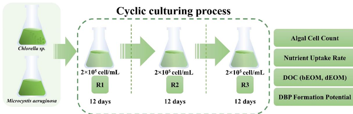
Fig. 1 Algal culturing process with three cycles for *Chlorella* sp. and *M. aeruginosa*.
