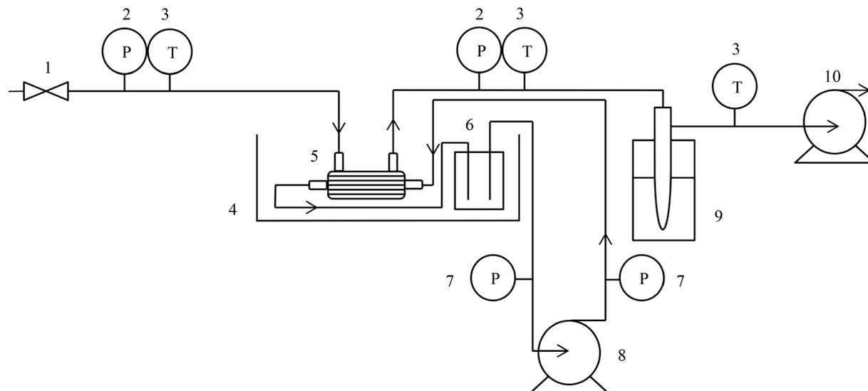
**Fig. 1** Membrane distillation and pervaporation membrane rig schematic. 1: Needle valve; 2: absolute pressure transducer; 3: temperature probe; 4: thermostatic bath; 5: membrane; 6: feed solution; 7: pressure gauge; 8: peristaltic pump; 9: liquid nitrogen cold trap or condenser; 10: diaphragm vacuum pump.
