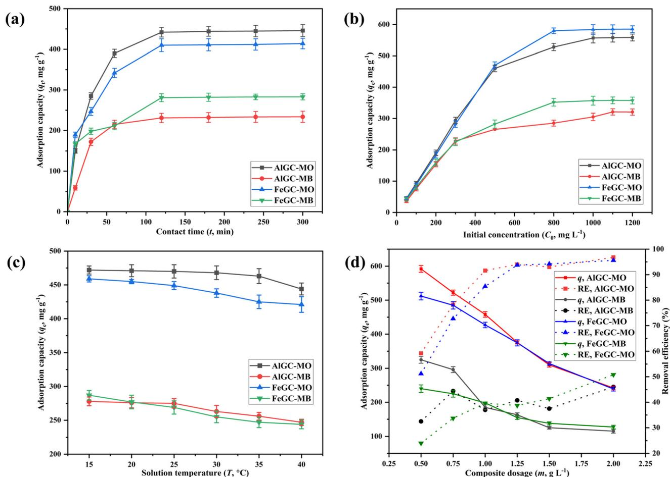
Fig. 14 Investigating the influence of (a)  $t$  (min), (b)  $C_0$ , (mg L<sup>-1</sup>), (c)  $T$  (°C), and (d)  $m$  (mg L<sup>-1</sup>) on MO and MB adsorption using AIGC and FeGC.
