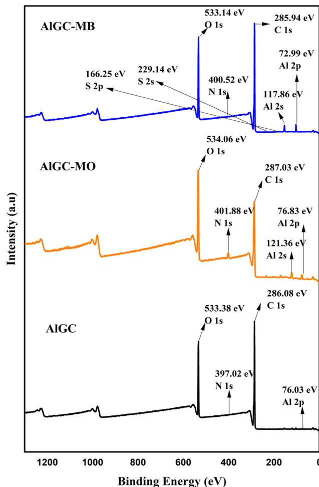
Fig. 9 The full XPS spectra of AlGC before and after dye adsorption.
