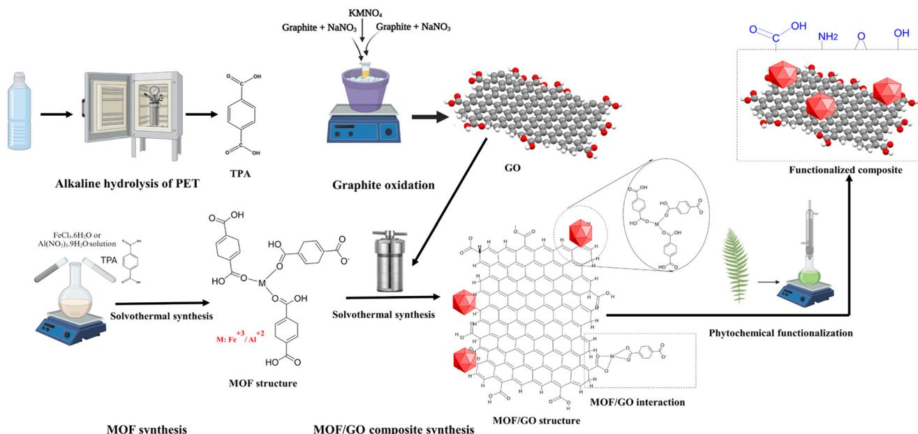
Fig. 1 Synthesis of the phytochemically functionalized GO/MOF composite.
