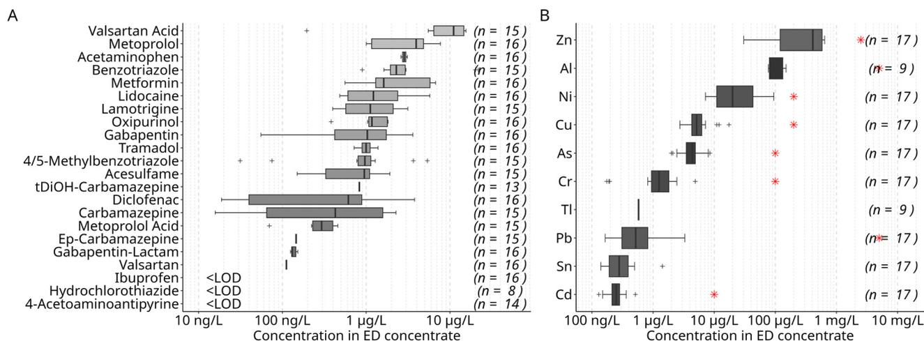
Fig. 6 Concentration of organic micropollutants (A) and metals and metalloids (B) in the electro dialysis concentrate derived as multi-nutrient solution by the nutrient recovery process ( $n$  = number of detects in 16 (A) and 17 (B) samples). Red crosses indicate the maximum concentration of metals and metalloids recommended for wastewater reuse.<sup>27</sup>
