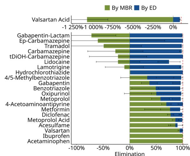
**Fig. 3** Calculated elimination in the membrane bioreactor and retention in the electrodiolysis of organic micropollutants aggregated across phase I and phase II. For individual compounds elimination, distinguished in both phases, is shown in Fig. 4. The dashed line indicates 100% elimination. The calculation of elimination is based on eqn (1).
