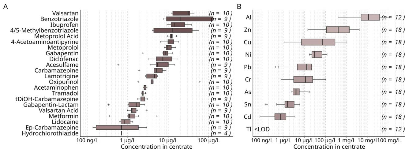
**Fig. 2** Median concentration of organic micropollutants (A) and metals and metalloids (B) in the centrate used as feed for the nutrient recovery process aggregated over the study period. Samples were obtained directly prior to treatment in the MBR ( $n$  = number of detects in 10 (A) and 18 (B) samples). Concentrations distinguished for phases I and II are shown in Table S7.†
