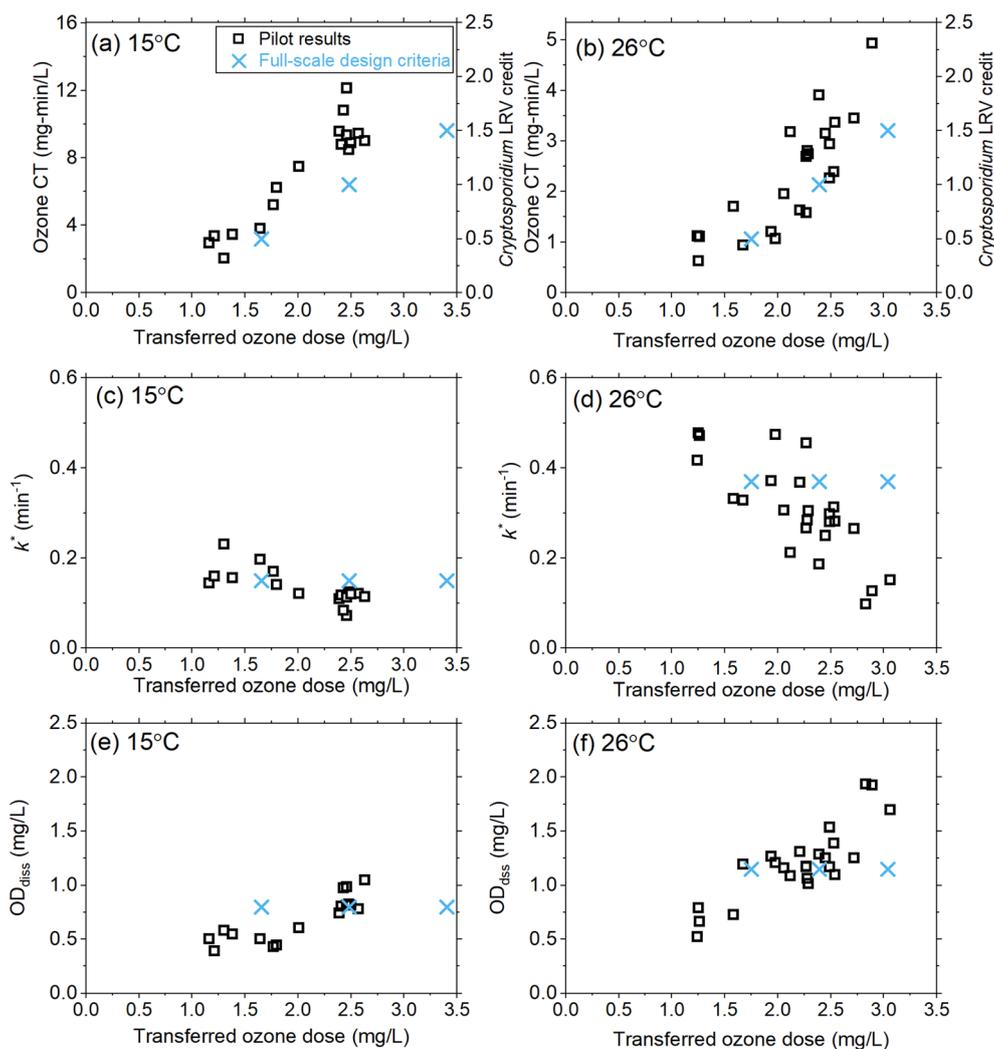
Fig. 6 Comparing pilot-scale results of this study to the initial full-scale design criteria at low ( $15\ ^\circ\text{C}$ , left panels) and high ( $26\ ^\circ\text{C}$ , right panels) design temperatures in terms of the effect of transferred ozone doses on (a and b) ozone CT (left y-axis) and LRV targets (right y-axis), (c and d)  $k^*$ , and (e and f)  $\text{OD}_{\text{diss}}$ .
