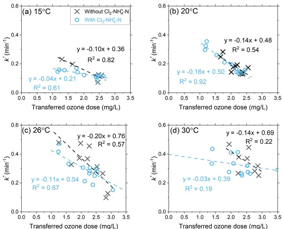
**Fig. 3** Pilot-scale data depicting the correlations between the first-order ozone decay rate constants as a function of the transferred ozone dose at (a) 15 °C, (b) 20 °C, (c) 26 °C, and (d) 30 °C. Pilot-scale results illustrating the different  $\text{Cl}_2\text{-NH}_4^+\text{-N}$  dosing scenarios are presented in Fig. S6†. Another representation of the data in terms of the effect of transferred ozone doses on ozone half-life for all tested temperatures is shown in Fig. S7†.
