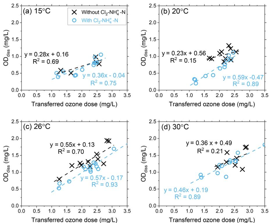
**Fig. 2** Pilot-scale data depicting correlations between  $OD_{diss}$  as a function of the transferred ozone doses at (a) 15 °C, (b) 20 °C, (c) 26 °C, and (d) 30 °C. Pilot-scale results illustrating the different  $Cl_2-NH_4^+-N$  dosing scenarios are presented in Fig. S5.†
