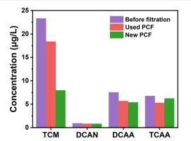
Fig. 6 DBPs changes in water treated by the new and used PCFs.
