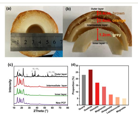
Fig. 1 (a) Cross-section photograph of the PCF, (b) photograph of different layers of the PCF, (c) XRD analysis of the used PCF and new PCF (G: goethite, Q: quartz, P: polypropylene,  $M_1$ : maghemite,  $M_2$ : magnetite), and (d) proportion of metal oxides in the PCF.
