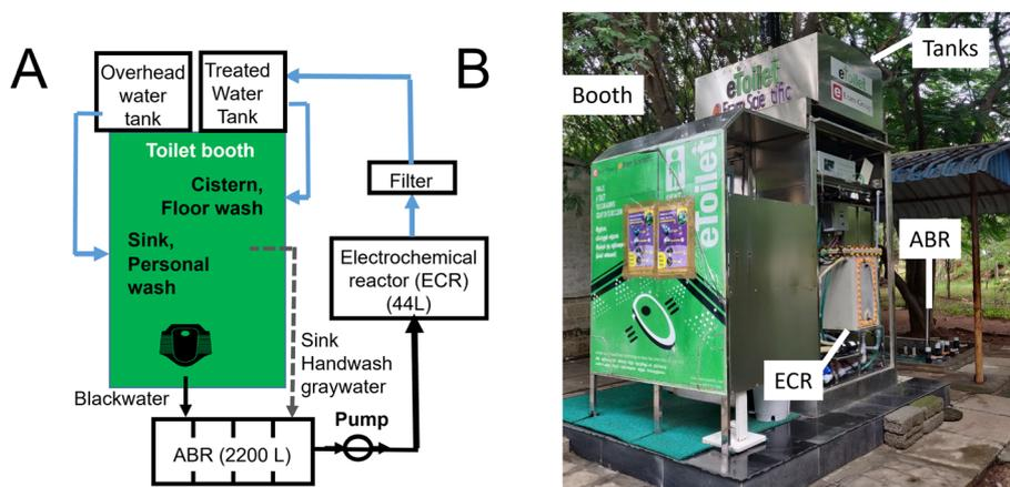
Fig. 1 A) Schematic of the apparatus. B) Picture of the system (doors of the ECR cabinet were removed to show the ECR tank).
