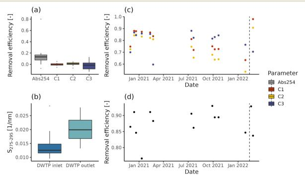
Fig. 2 Removal efficiency of organic matter (a) and the change of absorbance index S275-295 (b) in DWTP A (a and b), and temporal variations in organic matter removal in DWTP B (c and d) in terms of fluorescence (c) and absorbance (d).
