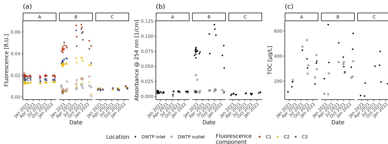
**Fig. 1** Intensity of fluorescent components C1, C2 and C3 (a), absorbance (b) and TOC (c) measured at the inlet and outlet of the monitored DWTPs (A–C) as a function of the sampling date. Closed and open markers indicate the DWTP inlet and outlet, respectively.
