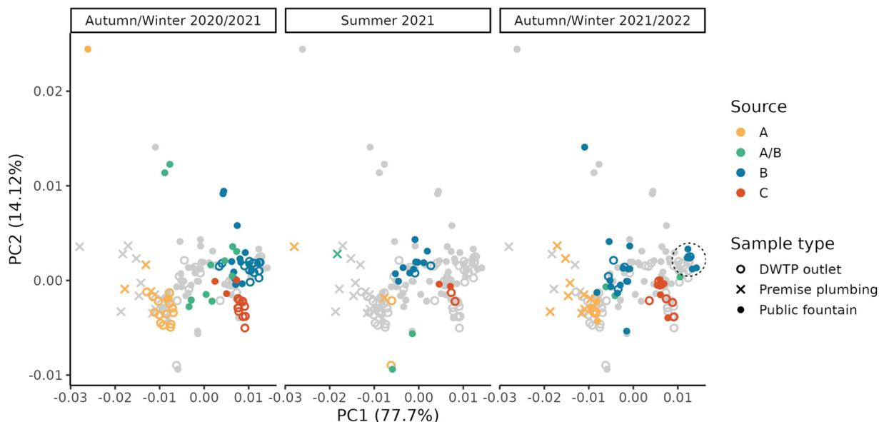
**Fig. 4** Principal component plot of the spectroscopic characteristics of the samples collected at the DWTP outlets and within the DWDN. The labels on the top of each panel indicate the period to which the coloured markers belong, while grey markers represent the samples collected in other seasons, in order to aid the comparison among facets. Markers inside the dashed circle indicate the samples from DWTP B collected after the activated carbon substitution.
