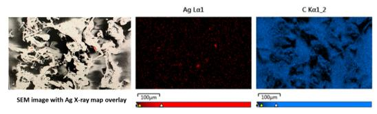
Fig. 5 SEM-EDS analysis of surface of 2%Ag abraded particles.
