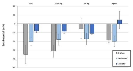
Fig. 6 Zeta potential (in mV) for the PETG, AgNP-PETG composites and AgNPs. Error bars represent ±1 standard deviations.
