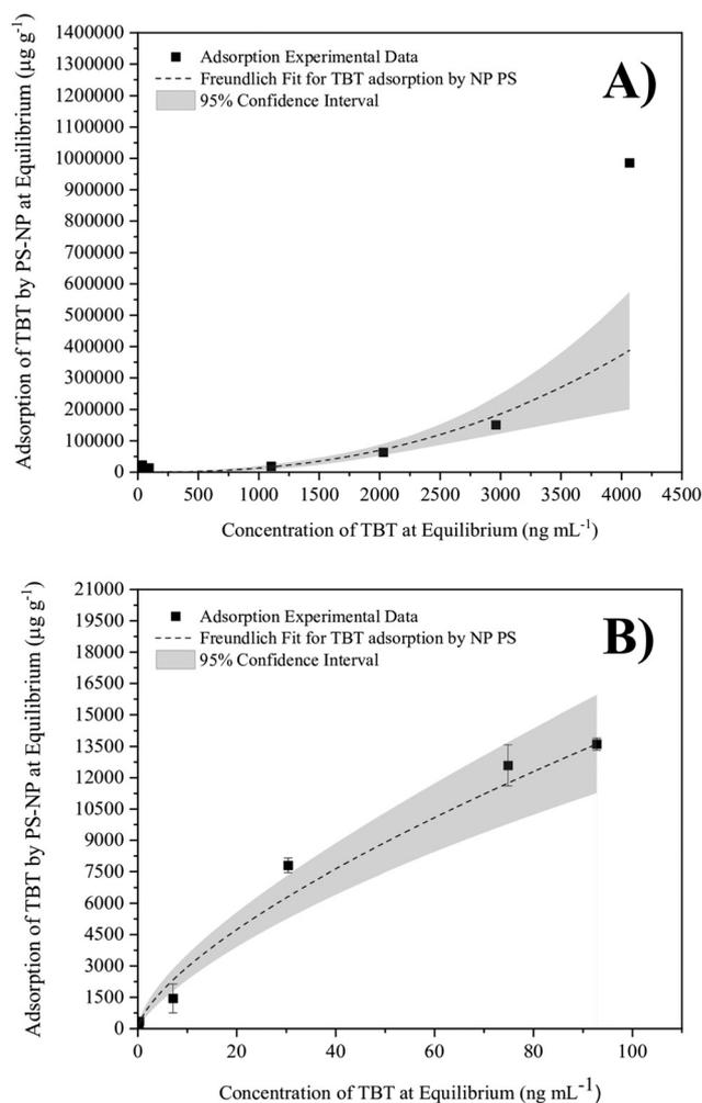
**Fig. 2** Adsorption of TBT by large PS-NP in pH 8 Milli-Q water, showing Freundlich fitting for TBT adsorption in phosphate pH 8 Milli-Q buffer across A) an extended concentration range and B) a concentration range limited by the TBT solubility limit.
