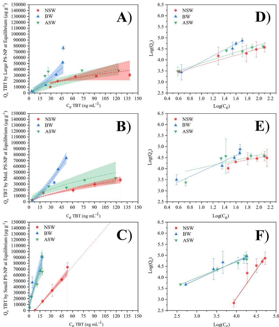
**Fig. 3** Freundlich fitting for TBT adsorption by varying size of polystyrene nanoplastic (large (A), medium (B), small (C)) in natural seawater (red circle), brackish water (blue triangle), and artificial seawater (green inverted triangle) across an environmentally occurring concentration range. Shaded regions display the 95% confidence intervals. Linearised Freundlich models for large (D) medium (E) and small (F) particles.
