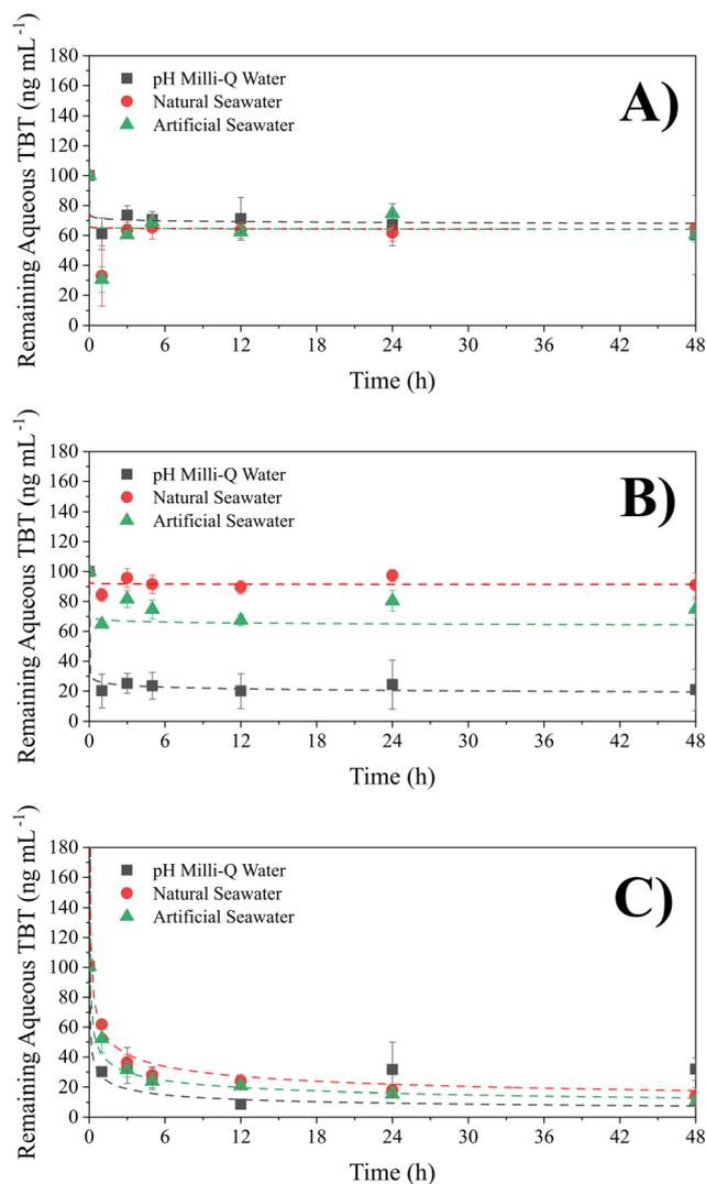
**Fig. 1** Kinetics of TBT adsorption by PS-NP, showing the relationship between aqueous TBT concentration ( $\text{ng mL}^{-1}$  TBT) and time (h) during kinetics experiments. A) Large PS-NP, B) medium PS-NP and C) small PS-NP. Experimental replicates are represented with error bars (SD,  $n = 3$ ).
