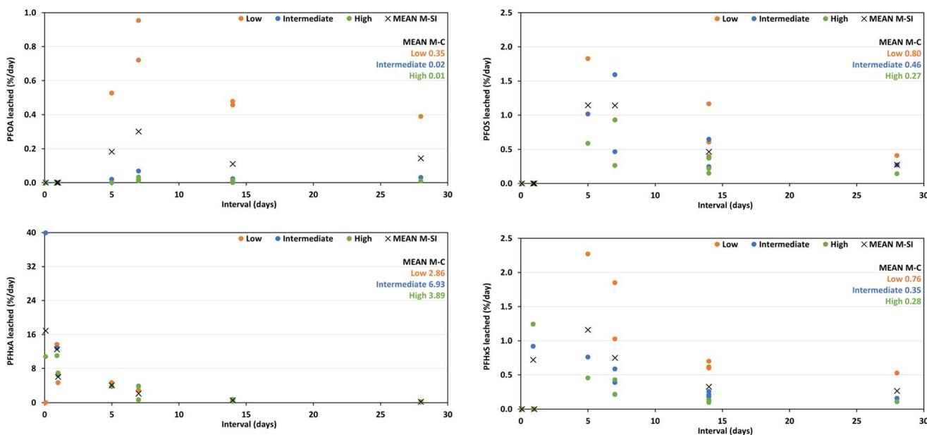
Fig. 5 The rate of PFAS leached (% d<sup>-1</sup>) from concrete monoliths at different sampling intervals. Mean M-SI represents the mean of the rate of PFAS leachability from concrete monoliths for three concentration levels at a given sampling interval. Mean M-C represents the mean of the rate of PFAS leachability for each concentration level of concrete monolith regardless of the sampling interval.
