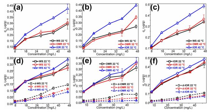
Fig. 2 Equilibrium sorption trends for the WS and treated soils at (a) 22 °C, (b) 32 °C, and (c) 42 °C; comparison of sorption and desorption trends at varying temperatures for the (d) WS, (e) OMR, and (f) IOR soils.
