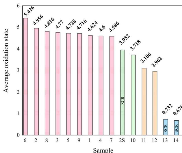
Fig. 6 Average selenium oxidation state for each sample.
