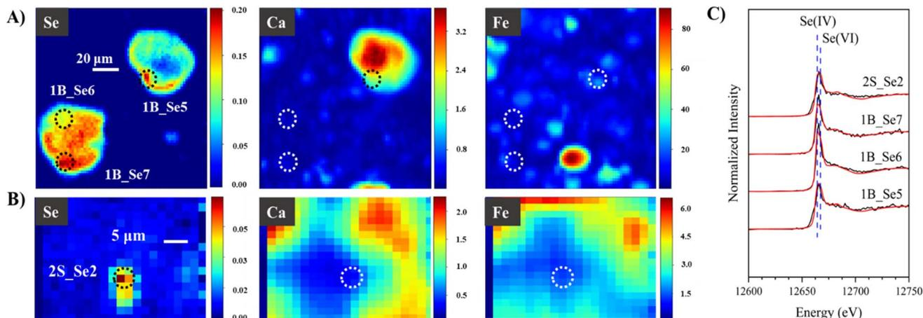
Fig. 3 Representative  $\mu$ -XRF elemental maps of Se, Ca, and Fe. (A) Hot spots 1B\_Se5, 1B\_Se6, and 1B\_Se7 for sample 1B. (B) Hot spot 2S\_Se2 for sample 2S. (C) Raw (black lines) and linear combination fitted  $\mu$ -XANES spectra (red lines) of the hot spots. Vertical dashed lines indicate the peak position for Se(IV) and Se(VI).
