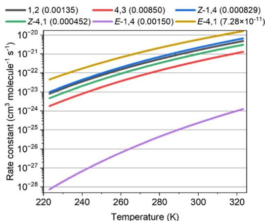
Fig. 3 Rate constants of the reaction of ISOPOOs + SO<sub>2</sub> to form ISOPOOSO<sub>2</sub>s for six isomers of ISOPOO. The value inside the parenthesis indicates the branching ratio of unimolecular reactions of ISOPOOSO<sub>2</sub>s to form SO<sub>3</sub>.
