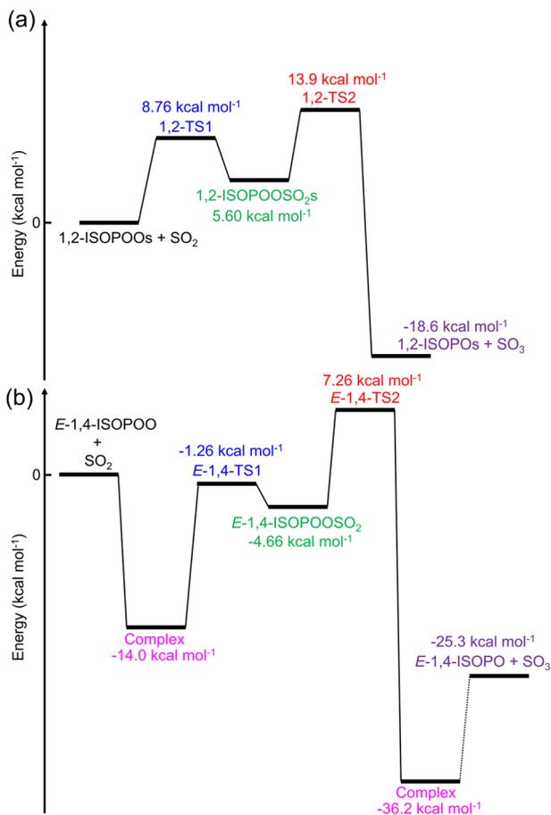
Fig. 2 Potential diagram of the entire ISOPOOs + SO<sub>2</sub> reaction obtained from the quantum chemical calculations for (a) 1,2-ISOPOO and (b) *E*-1,4-ISOPOO evaluated by CCSD(T)/aug-cc-pV(T+d)//M06-2X/aug-cc-pV(T+d)Z level of theory.
