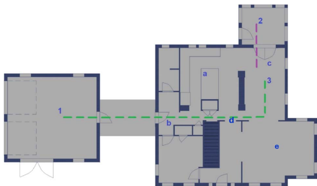
Fig. 2 NZERTF diagram of the first floor. Instruments were located in (1) the garage, (2) the enclosed porch, or (3) the dining room. Locations for (a) cooking, (b) aged smoke injection, (c) chemical cocktail, and (d) fresh smoke. The pesticide was sprayed in (e) the living room. Other chemicals, including ozone ( O_3 ), carbon dioxide ( CO_2 ), and ammonia ( NH_3 ), were injected directly into the supply air flow of the ventilation system (not shown). Dashed lines show sample lines from the garage (green) and porch (purple). Image created by Raleigh Robertson.
