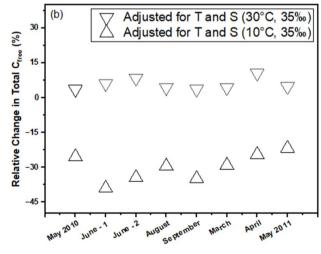
Fig. 7 Sum PAH of  $C_{\rm free}$  for eight sampling events. (a) Treatments include the  $C_{\rm free}$  adjusted for site specific temperature and salinity, the  $C_{\rm free}$  at an elevated temperature of 30 °C, and the  $C_{\rm free}$  at a reduced temperature of 10 °C. (b) The relative change in PAH  $C_{\rm free}$  at 30 °C and 10 °C compared to the actual station conditions.
