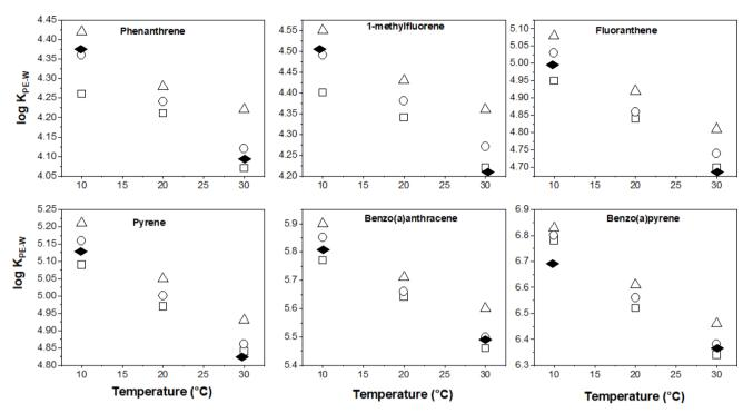
Fig. 2 Log  $K_{PE-W}$  versus temperature for selected PAHs as a function of salinity: ( $\square$ ) 0%, ( $\bigcirc$ )18%, and ( $\triangle$ ) 36% based on this investigation. For comparison, the black diamonds represent adjustments based on corrections reported by Lohmann (2012).
