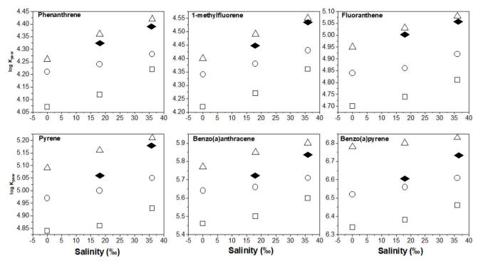
Fig. 5 Log  $K_{PE-W}$  – salinity correlation plots for selected PAHs as a function of temperature: ( $\triangle$ ) 10 °C, ( $\bigcirc$ ) 20 °C and ( $\square$ ) 30 °C based on this investigation. For comparison, the black diamonds represent adjustments based on corrections reported by Lohmann (2012).
