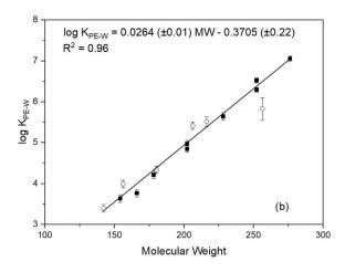
Fig. 1 Relationships between log  $K_{PE-W}$  and (a) molecular weight, (b) molecular volume, and (c) log  $K_{ow}$  for experimental system under standard conditions (20 °C, freshwater). Solid squares and open circles represent parent- and alkylated-PAHs, respectively, and the solid line represent the regression line. PAH consistently below the regression line (open circle) is 7,12 dimethyl benz[a]anthracene.
