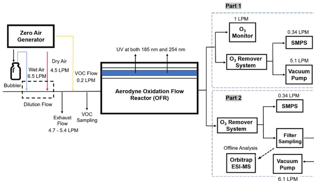
**Fig. 1** Schematic of the oxidation flow reactor. The experimental design used in this study which blue line, red line, and yellow line refer to wet air, dry air and VOC flow at the OFR inlet, respectively. Part 1 and part 2 at the OFR outlet are designed for different experiment purposes.
