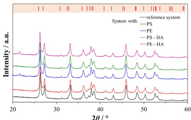
**Fig. 2** X-ray diffractograms of calcium carbonate samples precipitated in the reference system and with the addition of untreated and HA-treated PS and PE microspheres. The standard diffraction line positions of aragonite (red bars) are shown for comparison.
