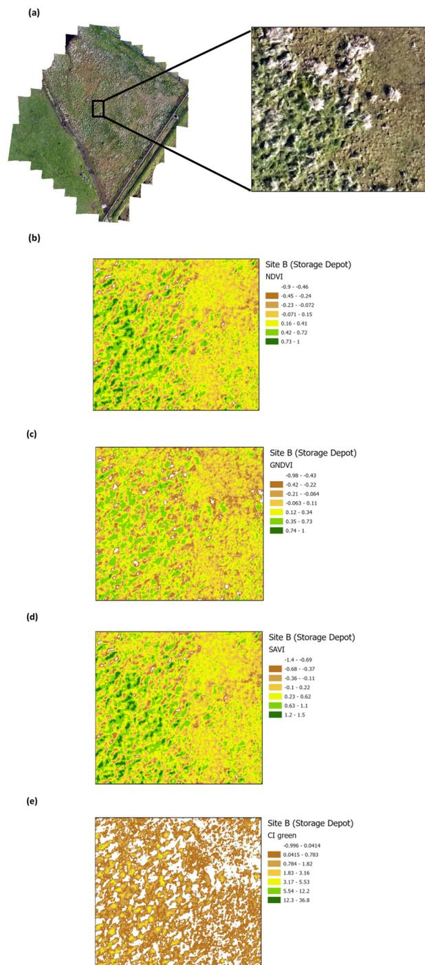
Fig. 8 Vegetation index maps for an area of Site B (Storage Depot) (a) RGB image indicating the area chosen from Site B (b) NDVI (c) GNDVI (d) SAVI and (e) CI green VI.
