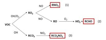
Fig. 5 The general VOC oxidation chemistry leading to the formation of key secondary pollutants: organic nitrates (RNO<sub>3</sub>), formaldehyde (HCHO) and PAN species (RCO<sub>3</sub>NO<sub>2</sub>).
