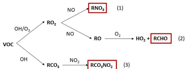
Fig. 5 The general VOC oxidation chemistry leading to the formation of key secondary pollutants: organic nitrates ( $\text{RNO}_3$ ), formaldehyde ( $\text{HCHO}$ ) and PAN species ( $\text{RCO}_3\text{NO}_2$ ).
