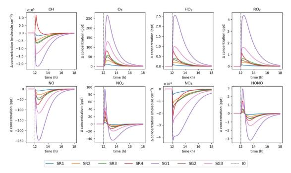
Fig. 4 Relative change in concentration of key indoor species from 11–18 h for each surface cleaner simulation, compared to a baseline simulation (no emissions).
