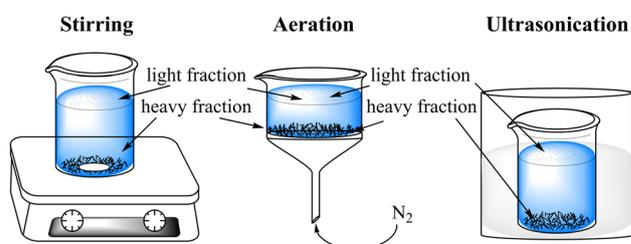
Fig. 1 Physical separation of contaminated soil in calcium chloride solution using stirring, aeration or ultrasonication. The calcium chloride solution was liquid–liquid extracted with 3  $\times$  40 mL dichloromethane (DCM, 99%, Sigma-Aldrich, Germany). The heavy fraction was washed as the light fraction.
