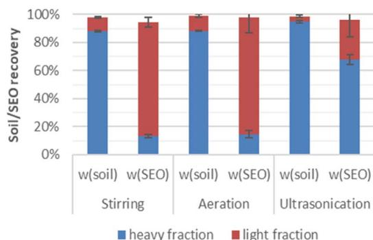
Fig. 2 Mass and SEO distributions in the light and heavy fractions after physical separation through stirring, aeration or ultrasonication in 39%  $\text{CaCl}_2$  solution ( $\rho = 1.40 \text{ g cm}^{-3}$ ).
