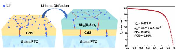
**Heterojunction lithiation engineering and diffusion-induced defect passivation for highly efficient Sb₂(S,Se)₃ solar cells**
