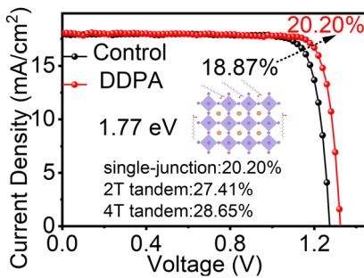
**Efficient 1.77 eV-bandgap perovskite and all-perovskite tandem solar cells enabled by long-alkyl phosphonic acid**
