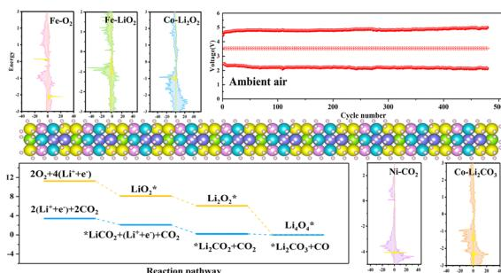
**A high-entropy cathode catalyst with multiphase catalytic capability of Li₂O₂ and Li₂CO₃ enabling ultralong cycle life in Li-air batteries**
